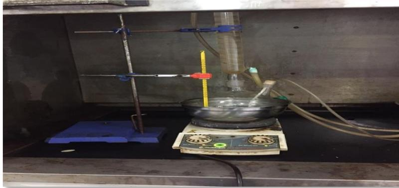
**Figure 3 Experimental device of ODS reactions**
