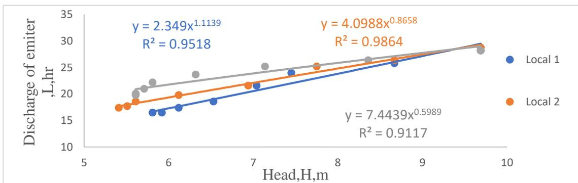
**Figure 4** The pressure-discharge relationship for products at pressure 1bar and emitter 1.
