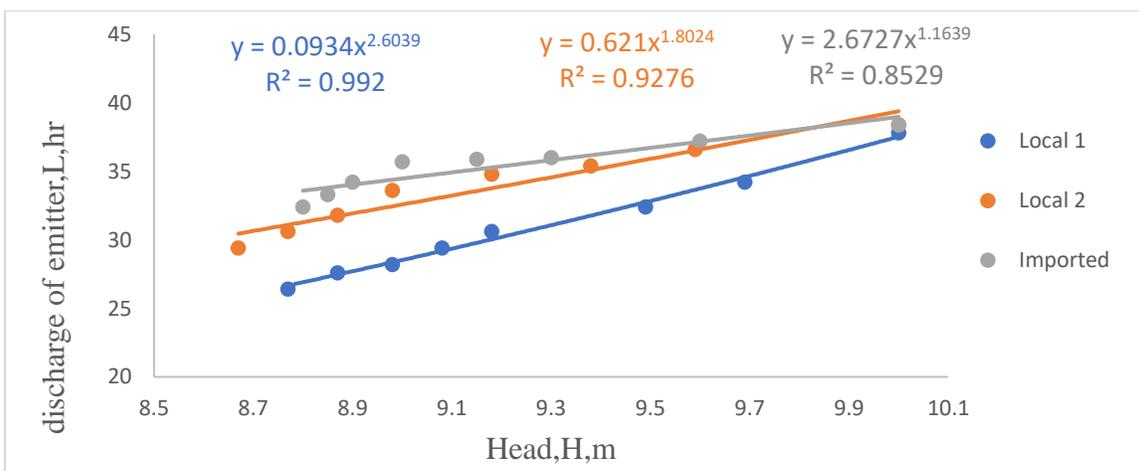
**Figure 5** The pressure-discharge relationship for products at pressure 1 bar and emitter 2.
