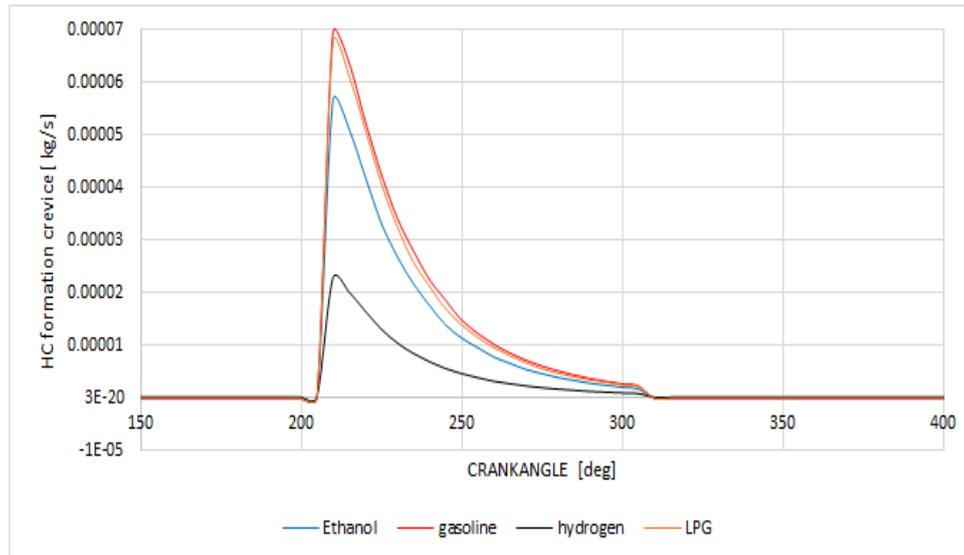
**Figure 5 Variation in HC formation of crevice with crank angle.**
