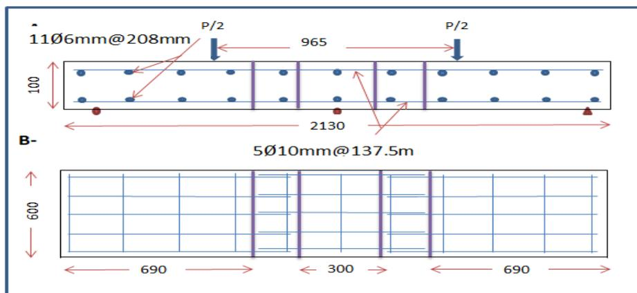
**Figure 6: Details of spliced specimen: A) Side view and B) Top view.**
