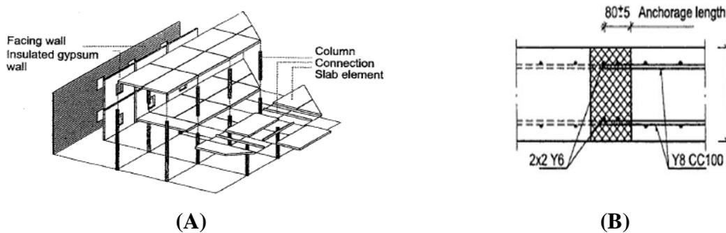
**Figure 1 A) Sketch of new building and B) Details of joint [1].**
