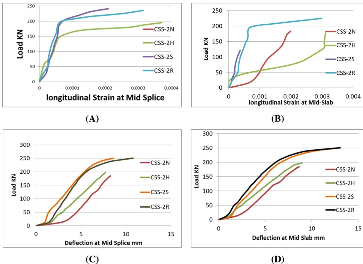
**Figure 13 Load-deflection and load-strain at :A) Longitudinal strain at mid splice, B) Longitudinal strain at mid slab, C) Deflection at mid splice, and D) Deflection at mid slab.**
