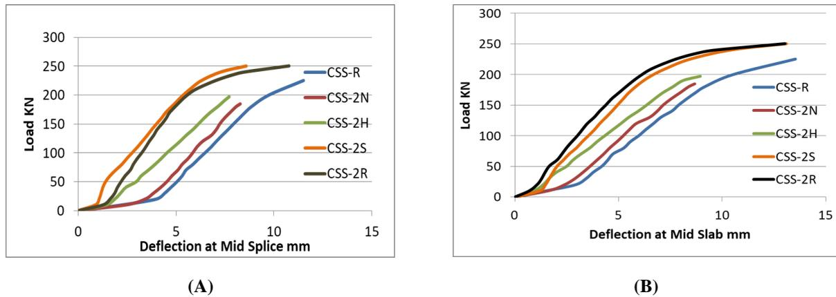
**Figure 9 Load-deflection curve at A) Deflection at mid splice and B) Deflection at mid slab.**
