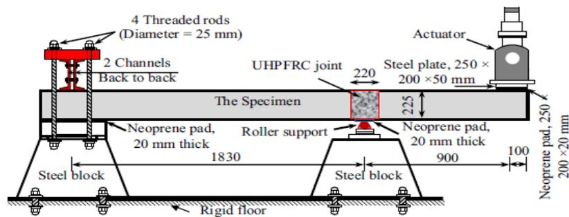
Figure 3 Details of specimen dimensions and support [4].
