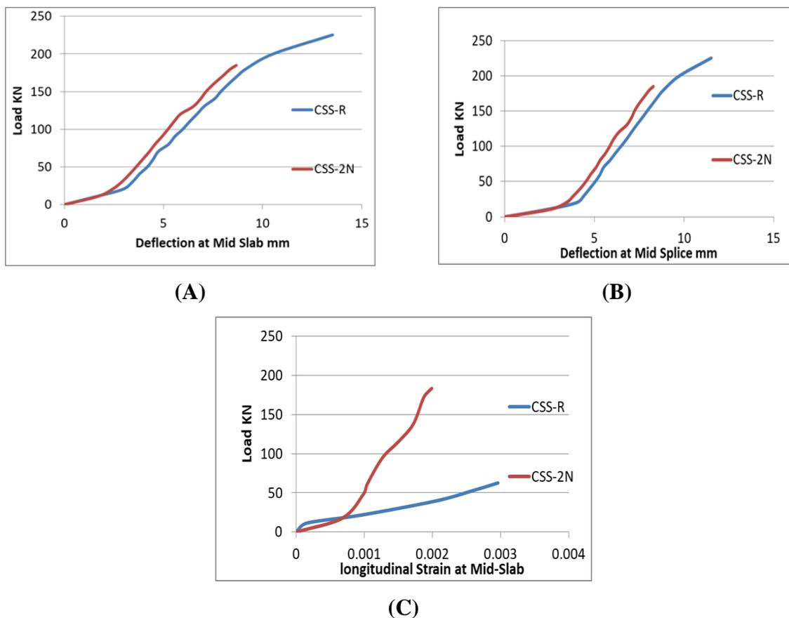
**Figure 12 The relationship between load-deflection and load-strain: A) deflection at mid slab, B) Deflection at mid splice, and C) Longitudinal strain at mid slab.**
