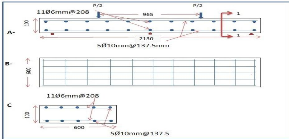
**Figure 5 Details of reference specimen A) Side view, B) Top view, and C) Section1-1.**
