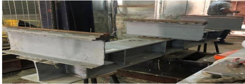
**Figure 8 Support fixed on the girder.**
