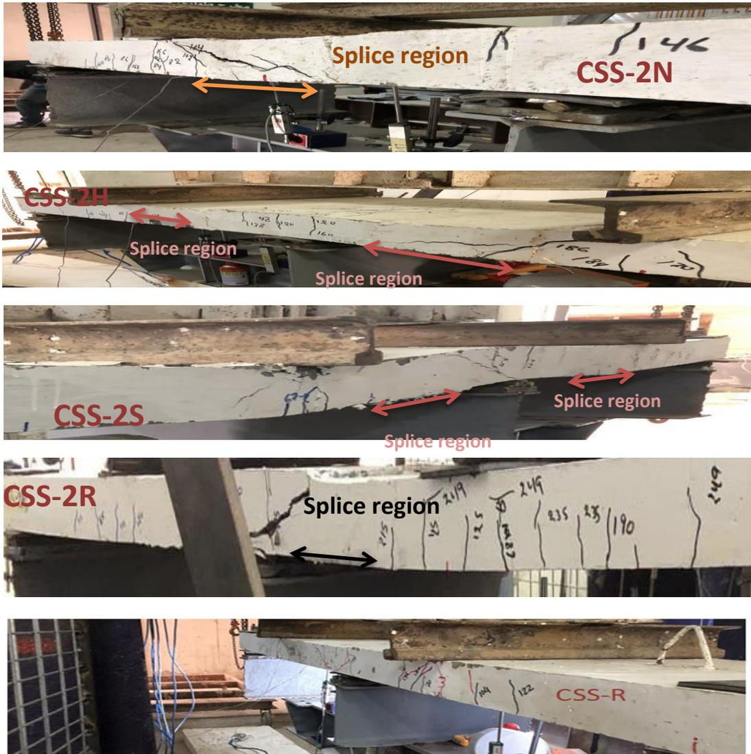
**Figure 10 Failure mode in continuous support one-way slab.**
