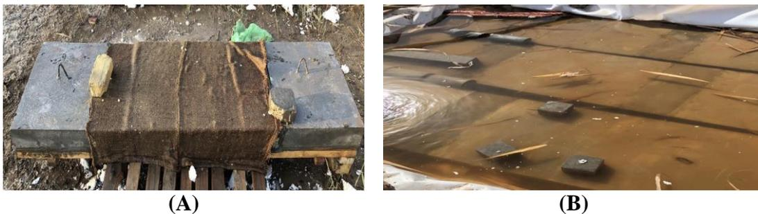
**Figure 7 A) Curing of specimens at normal temperature and B) Curing of specimen with RPC in the splice region.**
