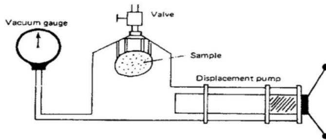
**Figure 2 Mercury injection pump[21]**
