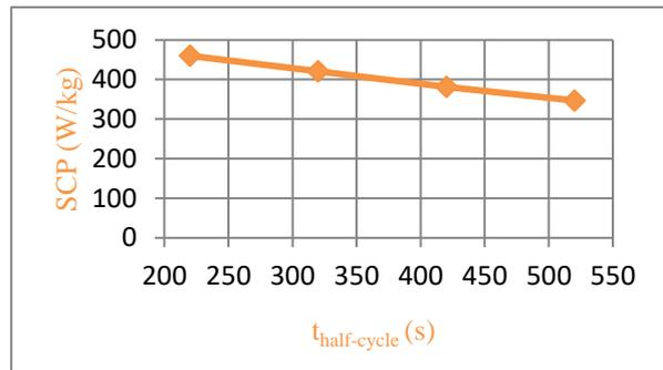
**Figure 11 Effect of half cycle time on SCP**
