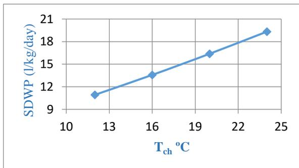
**Figure 6 Effect of evaporator water temperature on SDWP**
