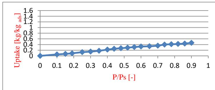
**Figure 5 Isotherms of Silica - gel at 25°C.**
