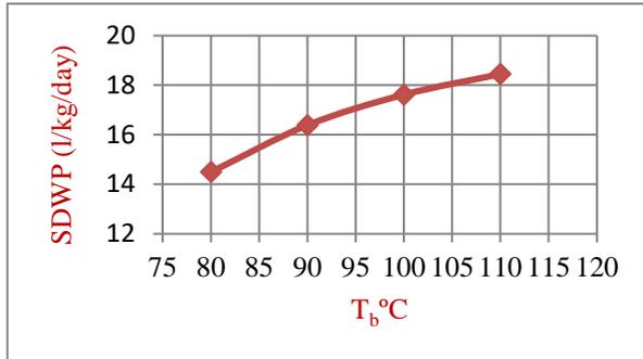
**Figure 3 Temperature of bed hot water effect on SDWP**
