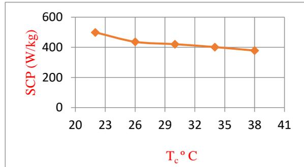
**Figure 9 Effect of condenser water temperature on SCP**
