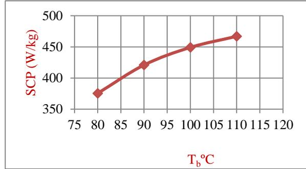
**Figure 4 Temperature of bed hot water effect on SCP**
