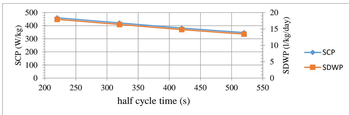
**Figure 12 SDWP & SCP of 2-beds cycle utilize silica-gel/water pair.  $T_{\text{b}}=90^{\circ}\text{C}$ ,  $T_{\text{c}}=30^{\circ}\text{C}$ ,  $T_{\text{ch}}=20^{\circ}\text{C}$**
