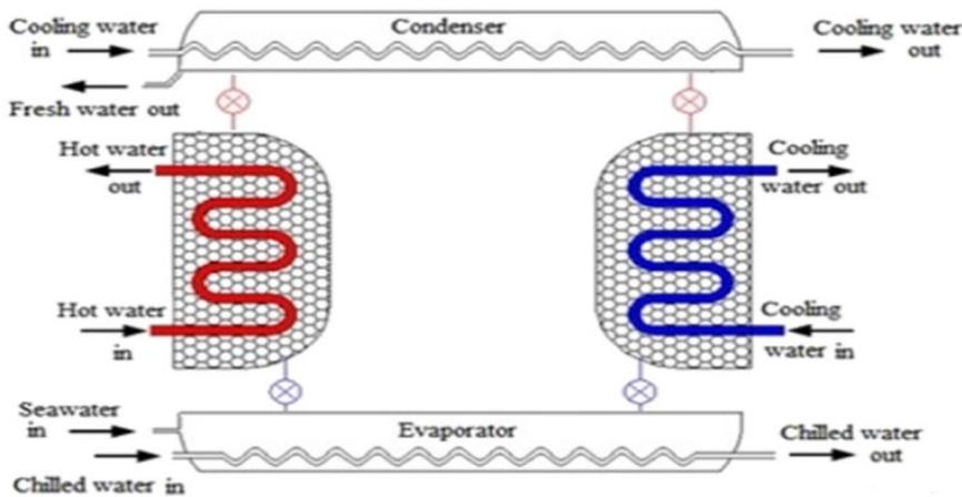
Figure 1 Schematic diagram of AD system[1].
