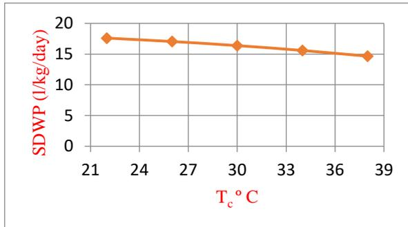
**Figure 8 Effect of condenser water temperature on SDWP**
