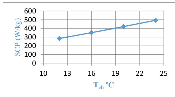
**Figure 7 Effect of evaporator water temperature on SCP**
