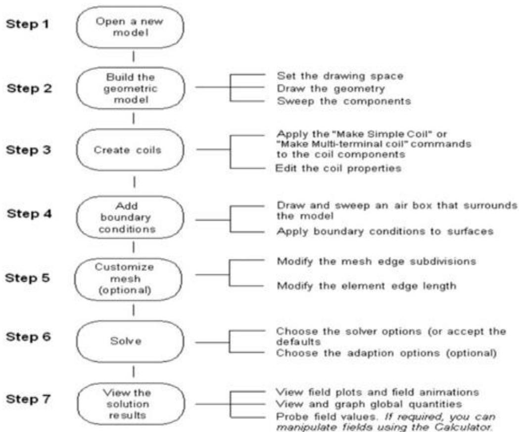
**Figure 1 Modeling steps by Magnet Software.**
