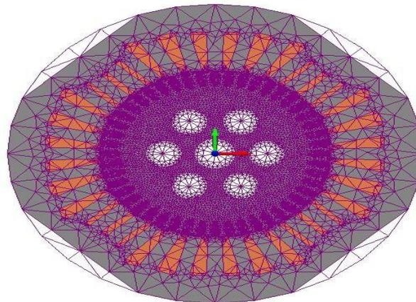
**Figure 6 Test motor model meshing by Magnet .**
