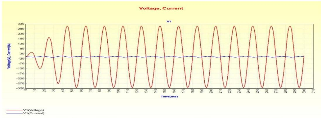
**Figure 7 Test motor rated voltage and current waveforms.**
