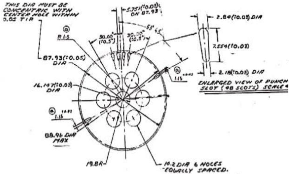
**Figure 5 rotor lamination of the test motor.**
