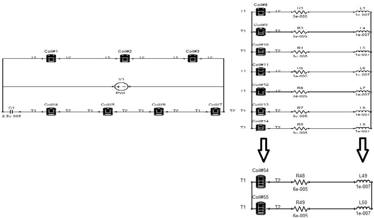
**Figure 2 The electric circuit of the test motor by Magnet.**
