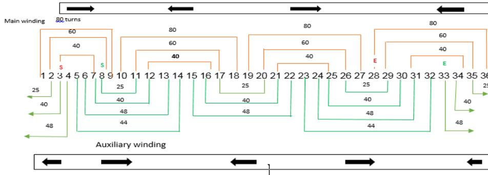
**Figure 3 Winding diagram of the test motor (arrows point to current direction).**
