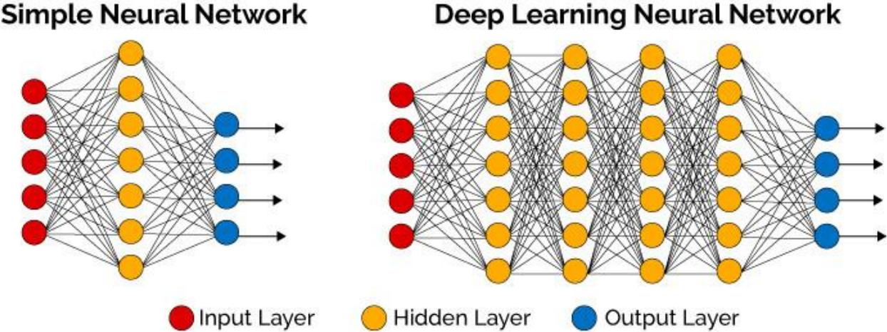
Figure 4. The architecture of Deep Neural Network [21]
