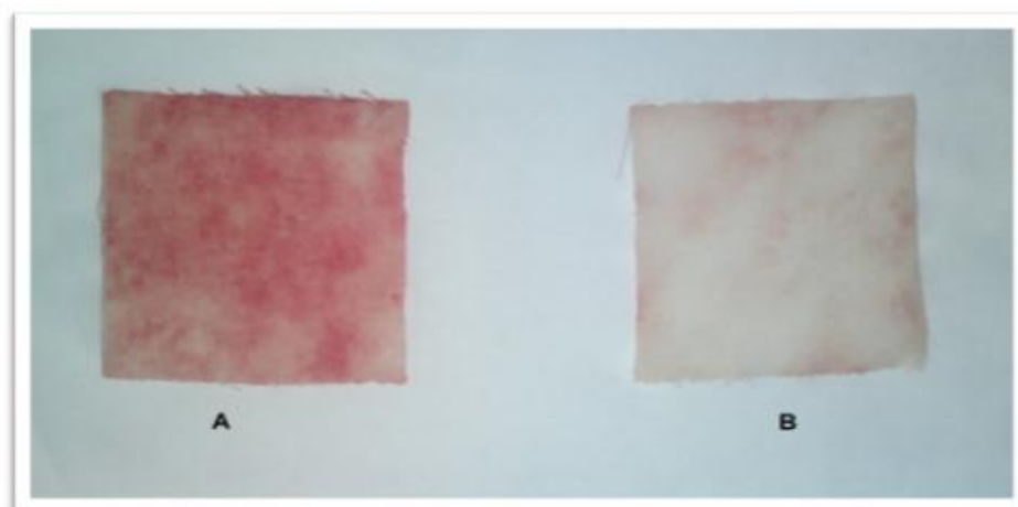
Figure (5): Removal of blood colors from cloth piece by crude protease of B. licheniformis B1. The blood-containing cloth piece was incubated with crude protease at 30°C for 30min. A, control (without enzyme); B, Sample treated with enzyme.
