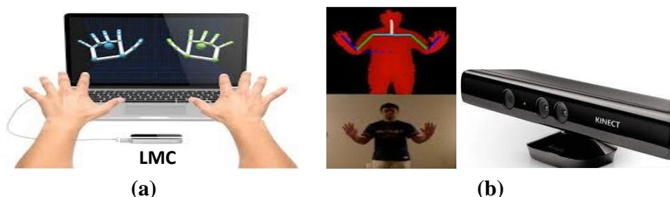
**Figure 5 (a) Leap motion controller (LMC), (b) Microsoft Kinect (MSK) [21].**
