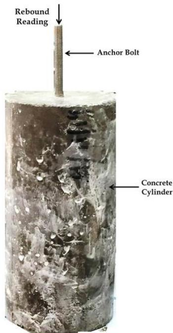
Figure 5. A view of a concrete cylinder with an embedded anchor bolt [4].
