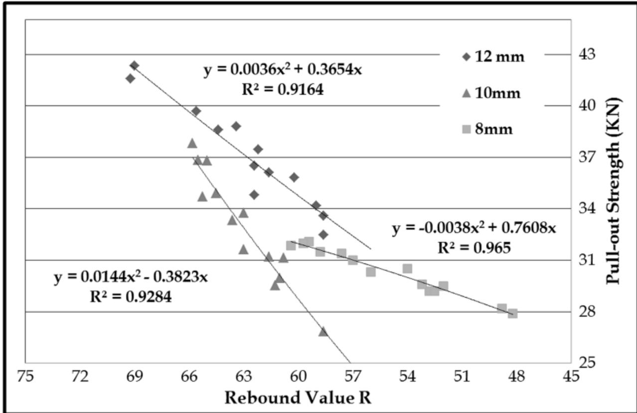
**Figure 8. Relationship between combined pull-out load and rebound value [4].**
