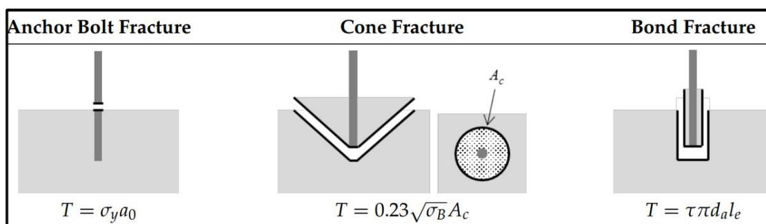
**Figure 1. Anchor bolts fracture modes [1].**
