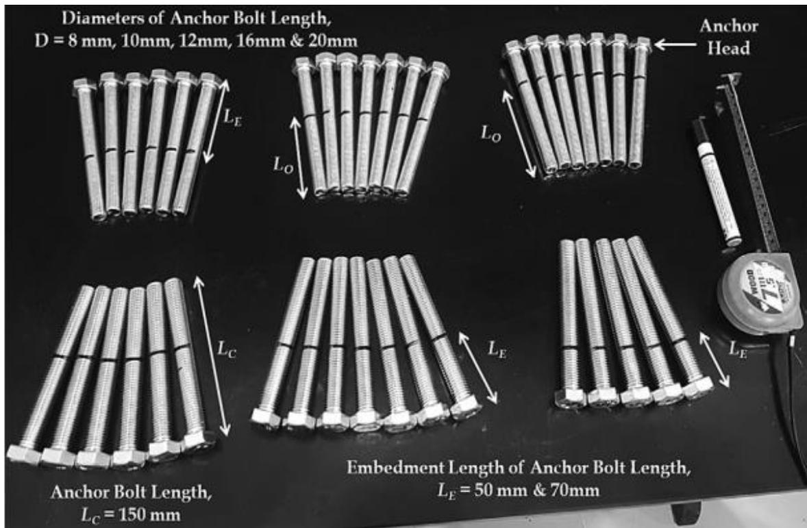
Figure 9. A view of used concrete anchor bolts in the study [5].
