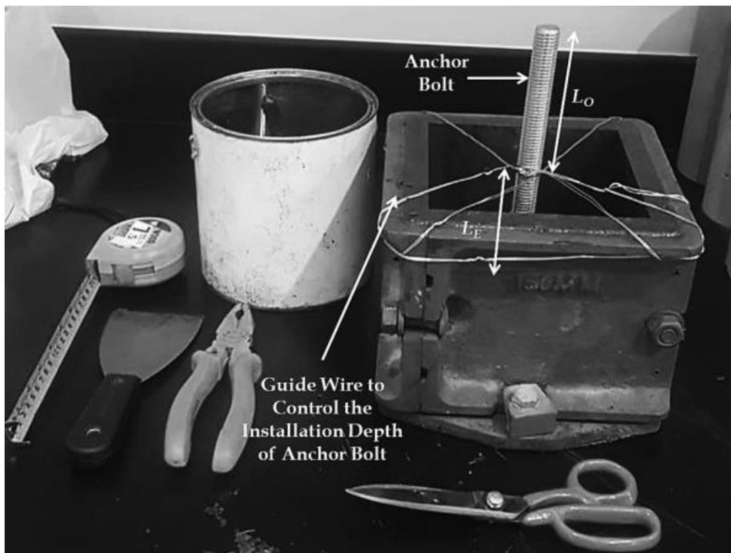
Figure 10. A view of the guide wire mechanism for steel Anchor bolt installation [5].
