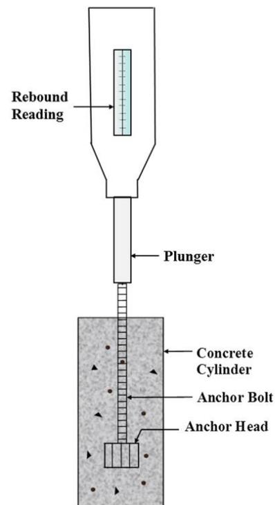
**Figure 3. Configuration of the experimental for recording the rebound value on the anchor bolt [3].**
