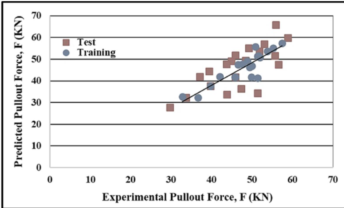
Figure 15. Comparison between the experimental pull-out force and the projected pull-out force using an MLP-5-4-1 neural network [35].
