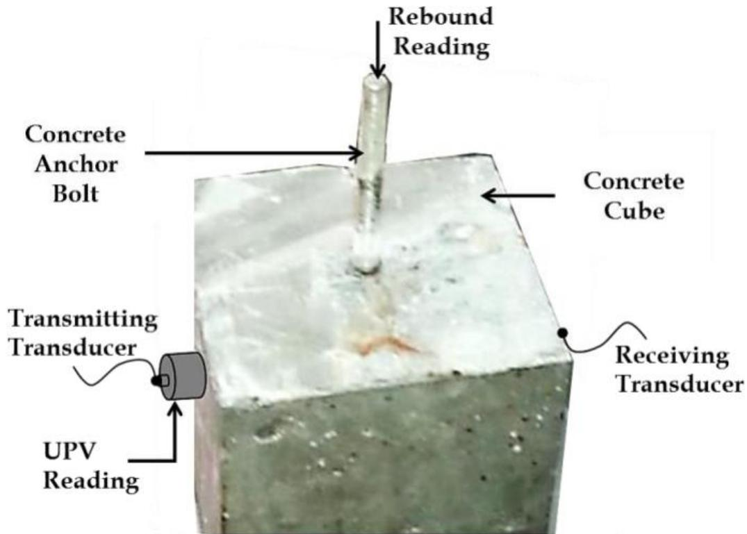
**Figure 13. Cube-shaped specimen illustrating Schmidt hammer and UPV testing [36].**
