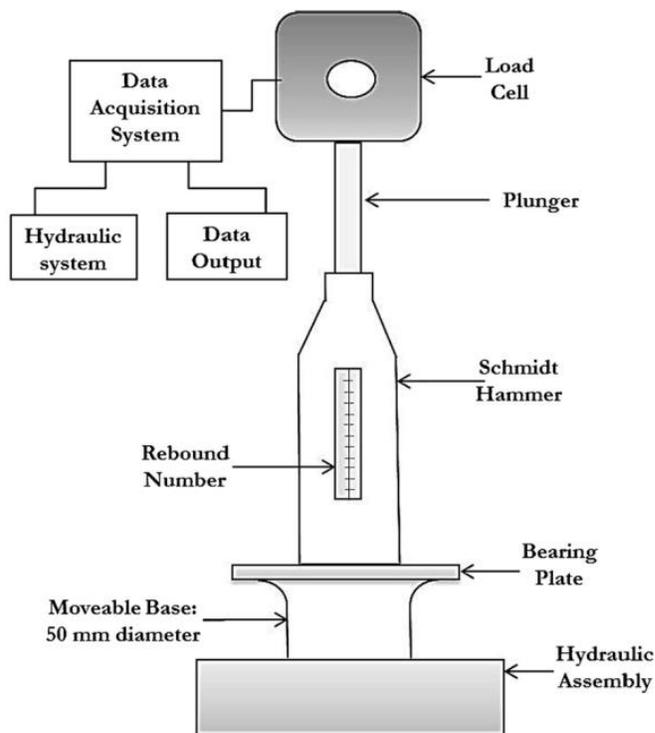
**Figure 2. The experimental set up for measuring the Schmidt hammer impact force [3].**
