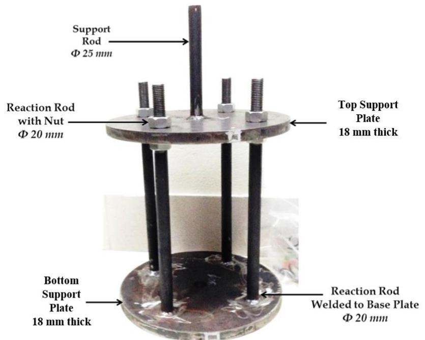
Figure 6. A view of the anchoring device [4].
