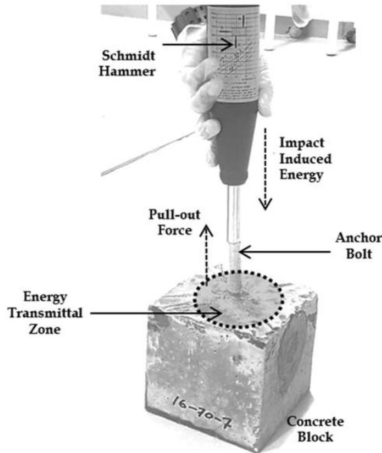
Figure 11. A View of the mechanism used for testing the cube specimens [5].
