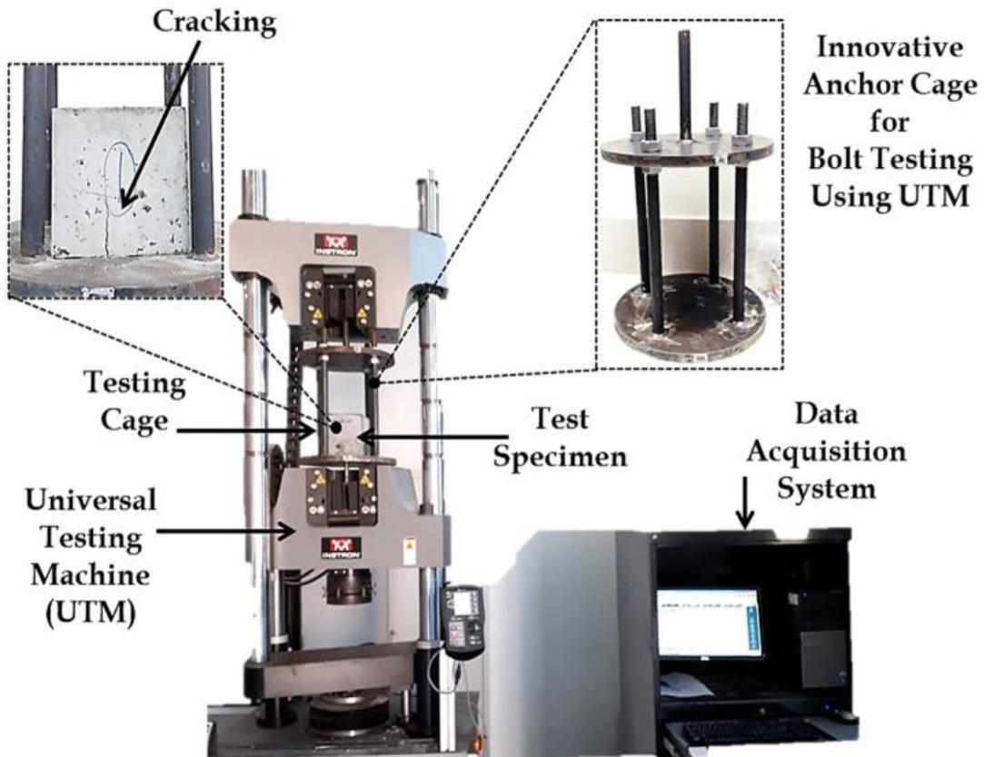
Figure 12. The test setup and anchor cage employed for the execution of pull-out testing with the Universal Testing Machine [5].
