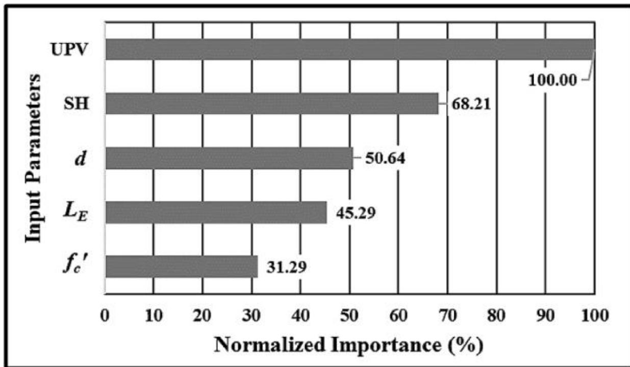
Figure 16. Normalized input parameter importance for MLP-5-4-1 [35].
