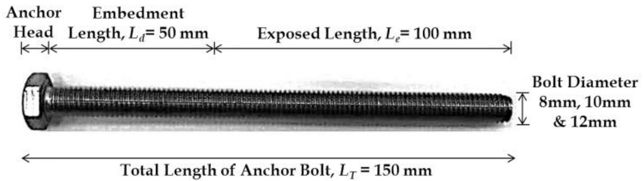
Figure 4. A view of the anchor bolt [4].
