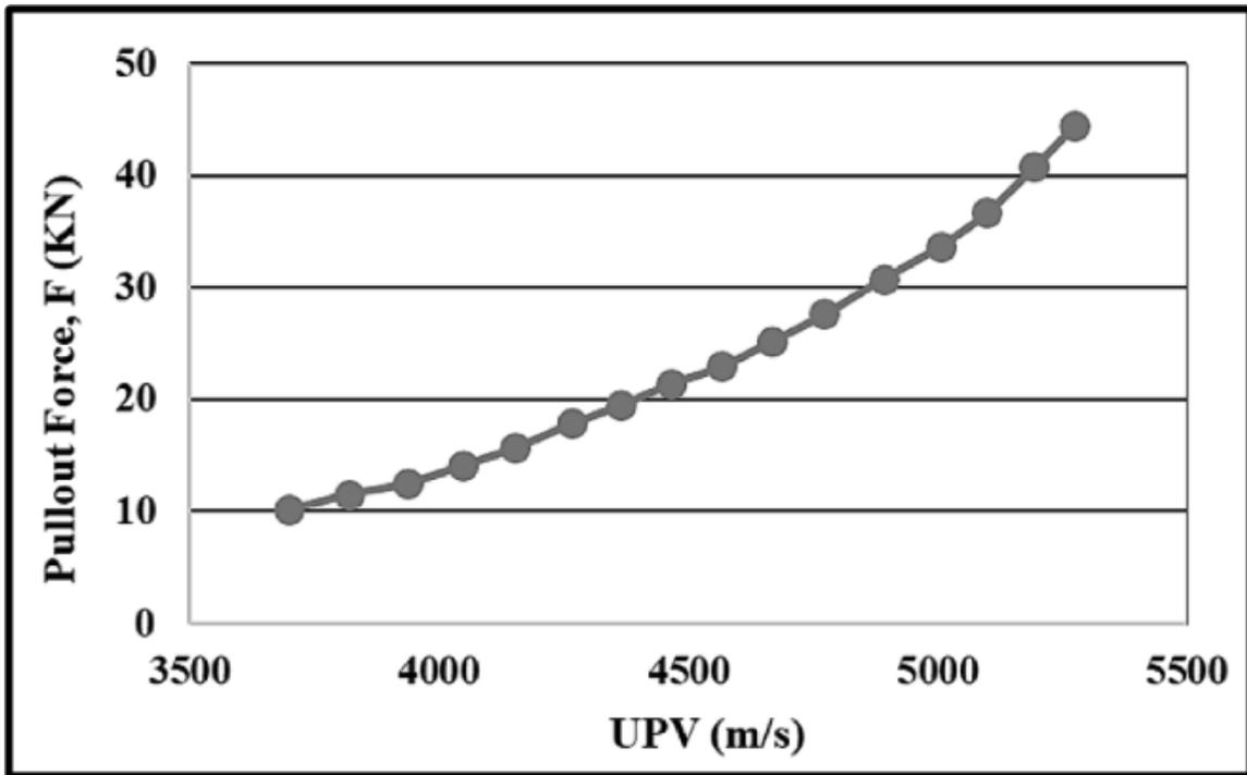
**Figure 17. The pull-out force of an embedded anchor bolt in concrete is examined concerning the UPV [35].**
