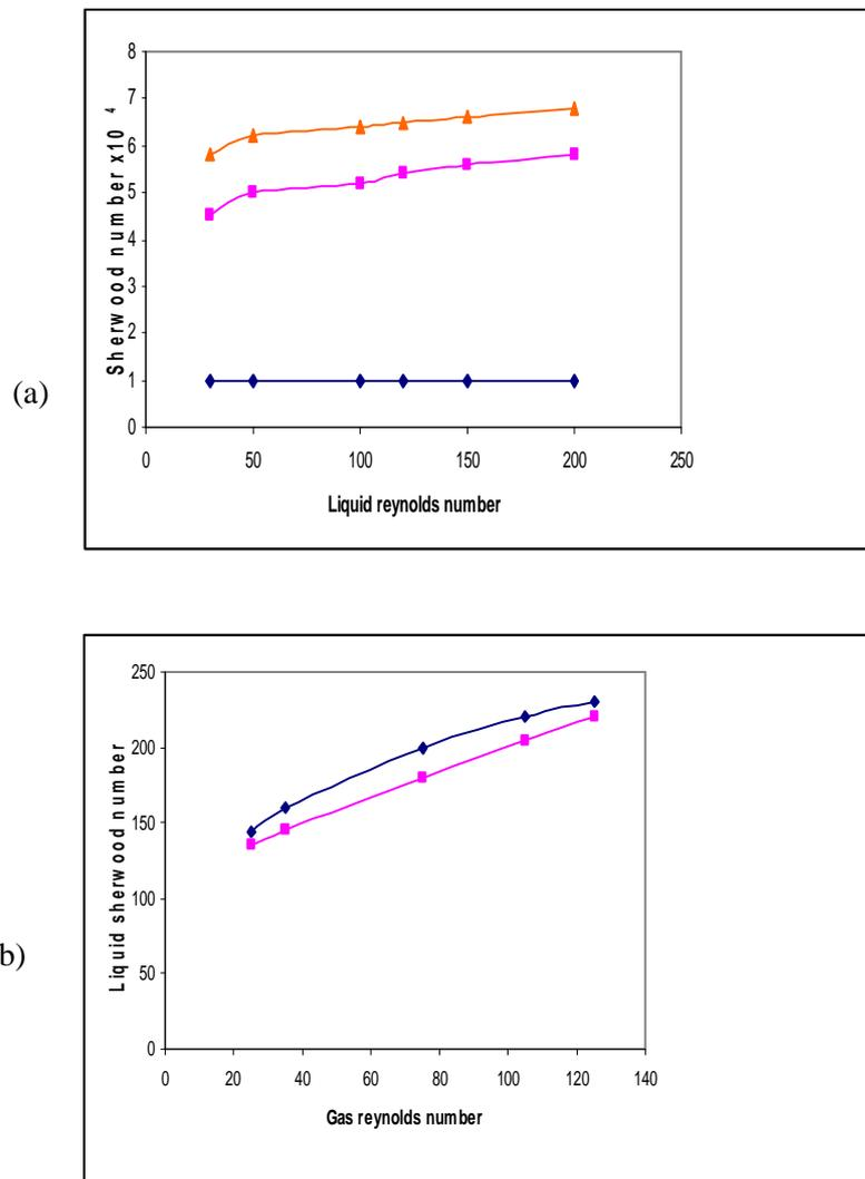
Figure (8) Liquid Reynolds number as function of Liquid Sherwood number with different gas flow rates
