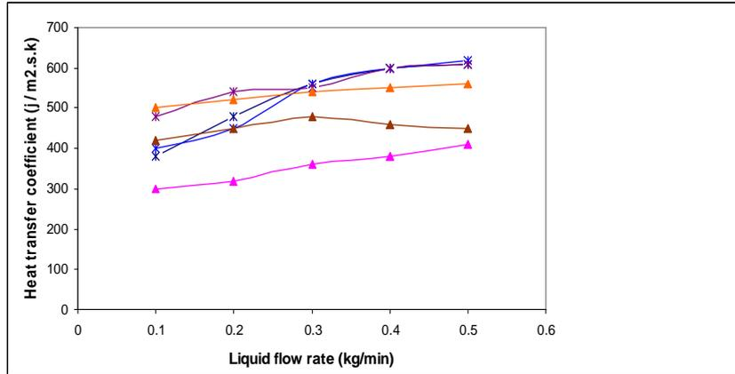
Figure (4) Effect of liquid flow rate on heat transfer Coefficient for different gas flow rates.
