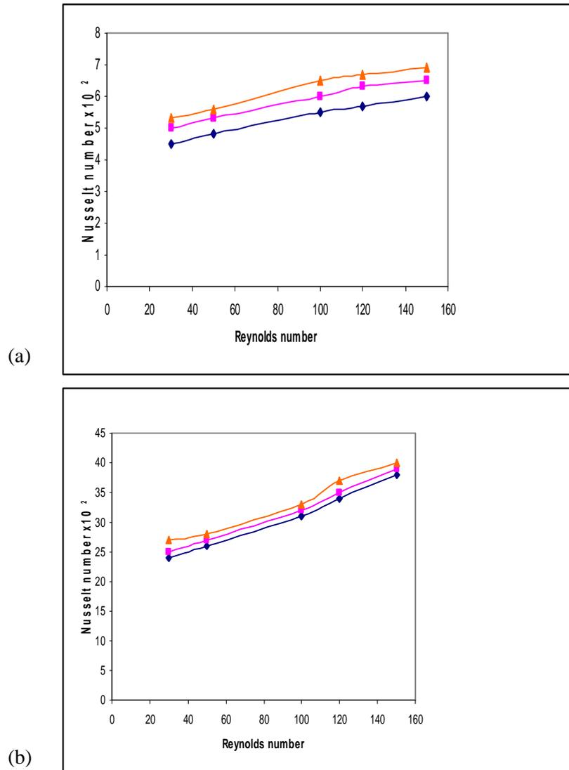
Figure (9) Liquid Reynolds number as function of Nusselt number different gas flow rates
