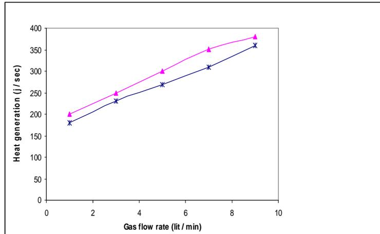
**Figure (6) Heat generation as function of gas flow rate, for liquid flow rate of 0.3 kg/ min and 40% concentration**
