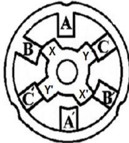
**Figure (1) cross section of a 6/4 SRM structure**
