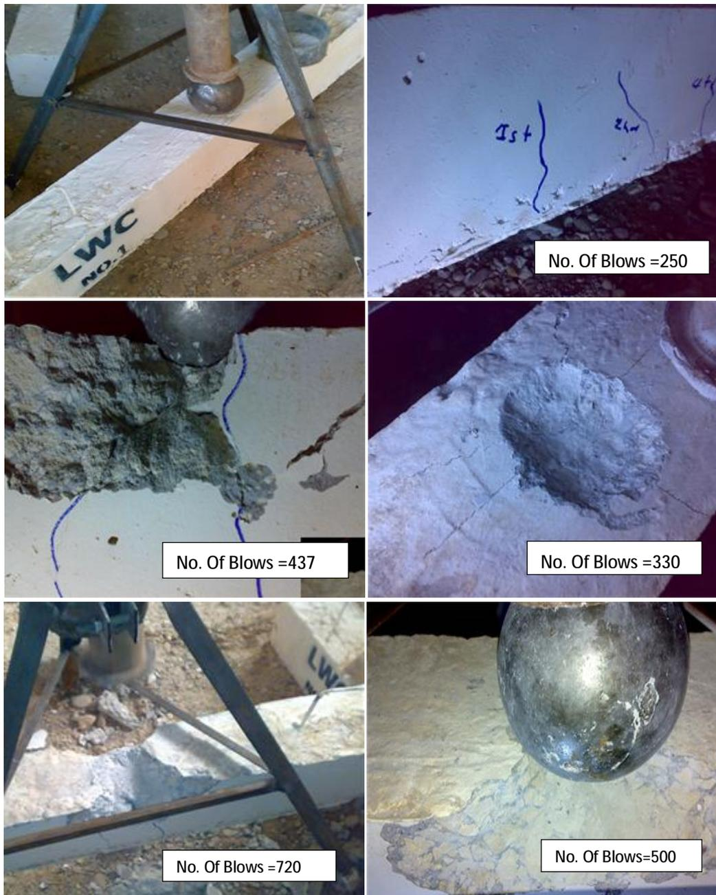
Figure (12) Number of blows from first crack up to failure for lightweight Concrete beam
