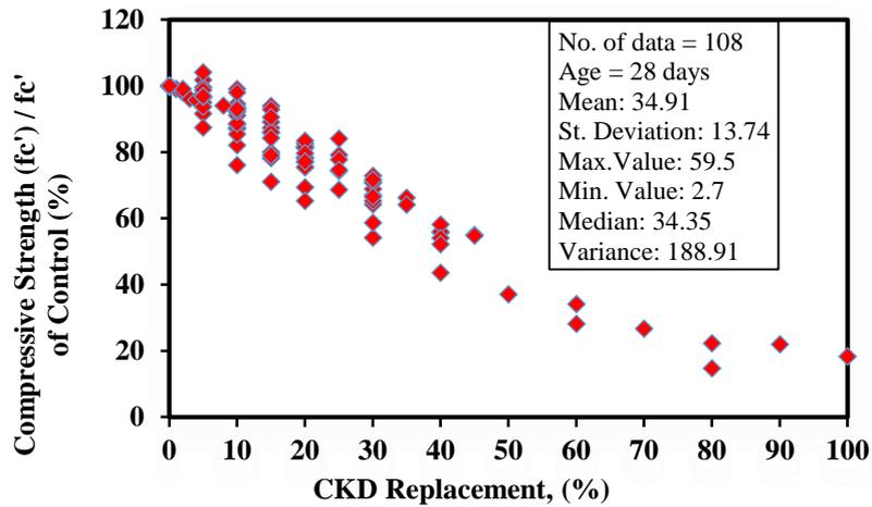
Figure 18. Statical Analysis of Compressive Strength at 28 Days, Collected from Table 1.
