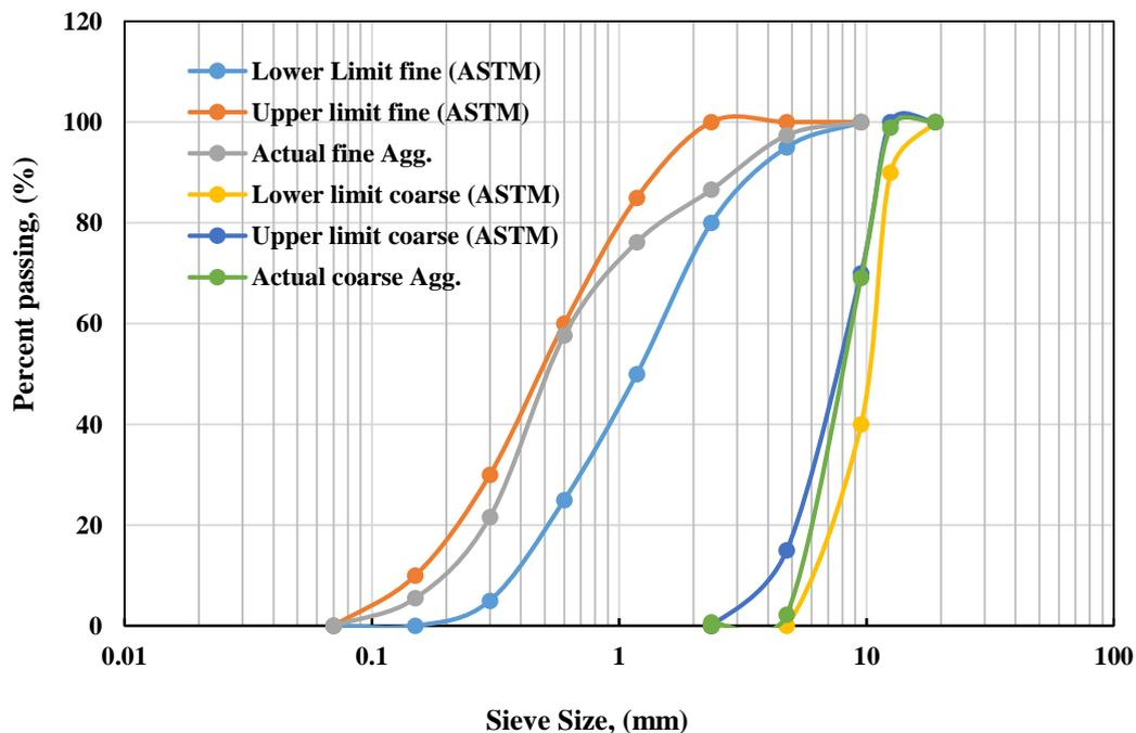
**Figure 6. Sieve Analysis of Fine and Coarse Aggregate According to ASTM C33 [24].**
