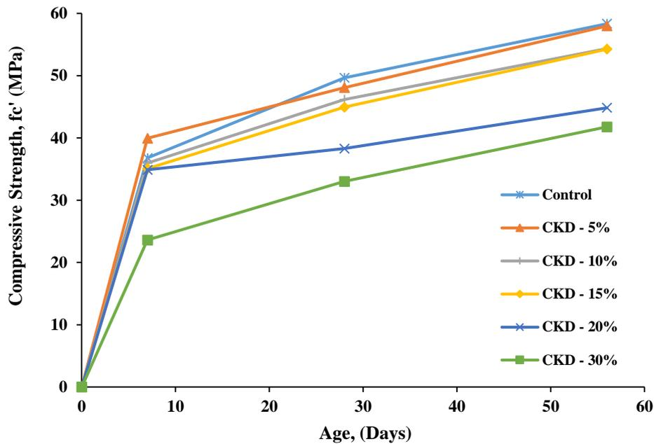
**Figure 13. Effect of CKD on Compressive Strength of the Concrete.**
