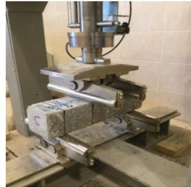
(b) Flexural Strength Machine Test.
