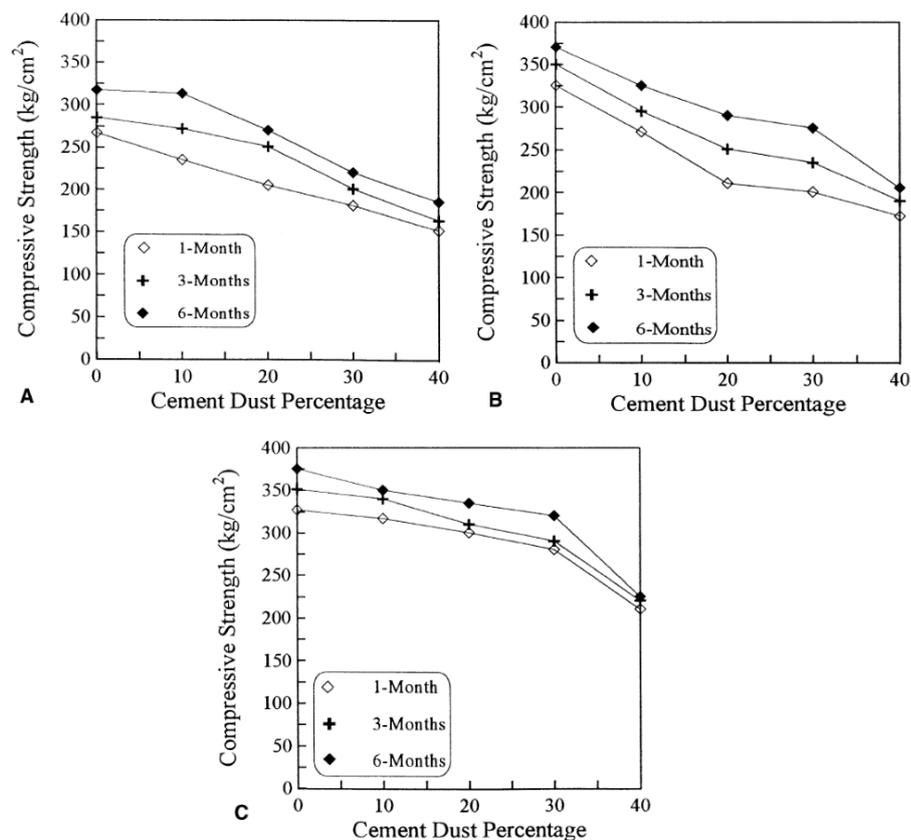
**Figure 3. Effect of CKD on compressive strength of concrete for different types of cement: A. CKD with OPC. B. CKD with BFSC. C. CKD with SRC [18].**
