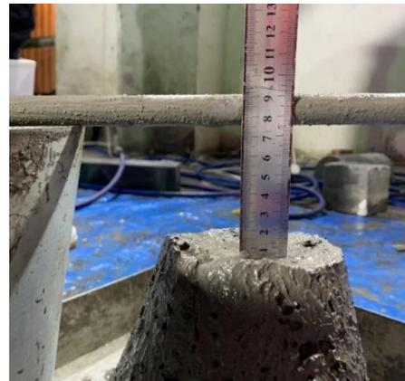
(b) Slump Test According to ASTM C143 [29].
