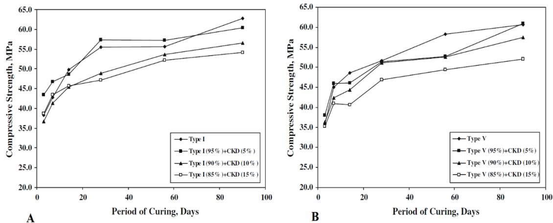
**Figure 4. Effect of CKD on two different types of cement: A. Type I of cement. B. Type V of cement [19].**
