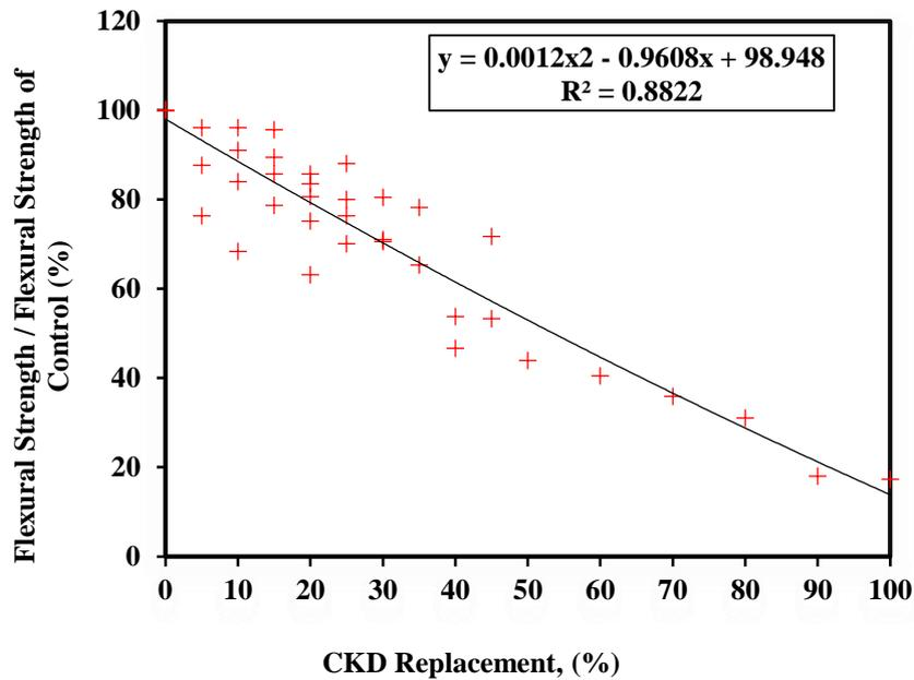
**Figure 22.** Non-Linear Regression of Flexural Strength at Age 28 Days.
