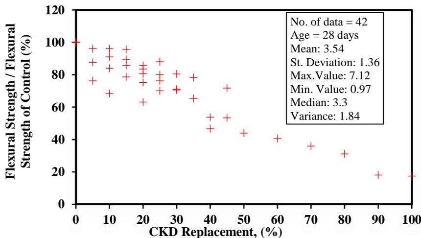
Figure 21. Statical Analysis of Flexural Strength at 28 Days, Collected from Table 1.
