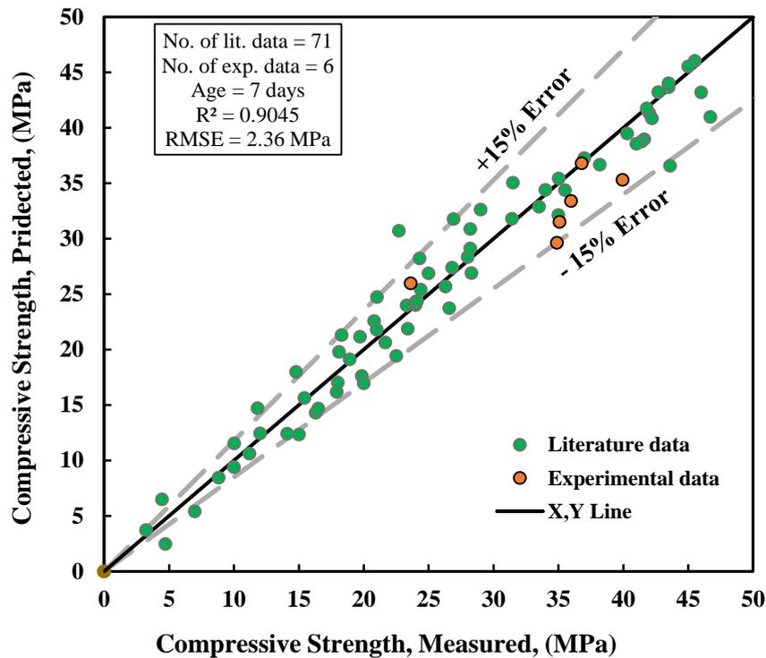
**Figure 17. Relation Between the Measured and Predict Compressive Strength at 7 Days.**
