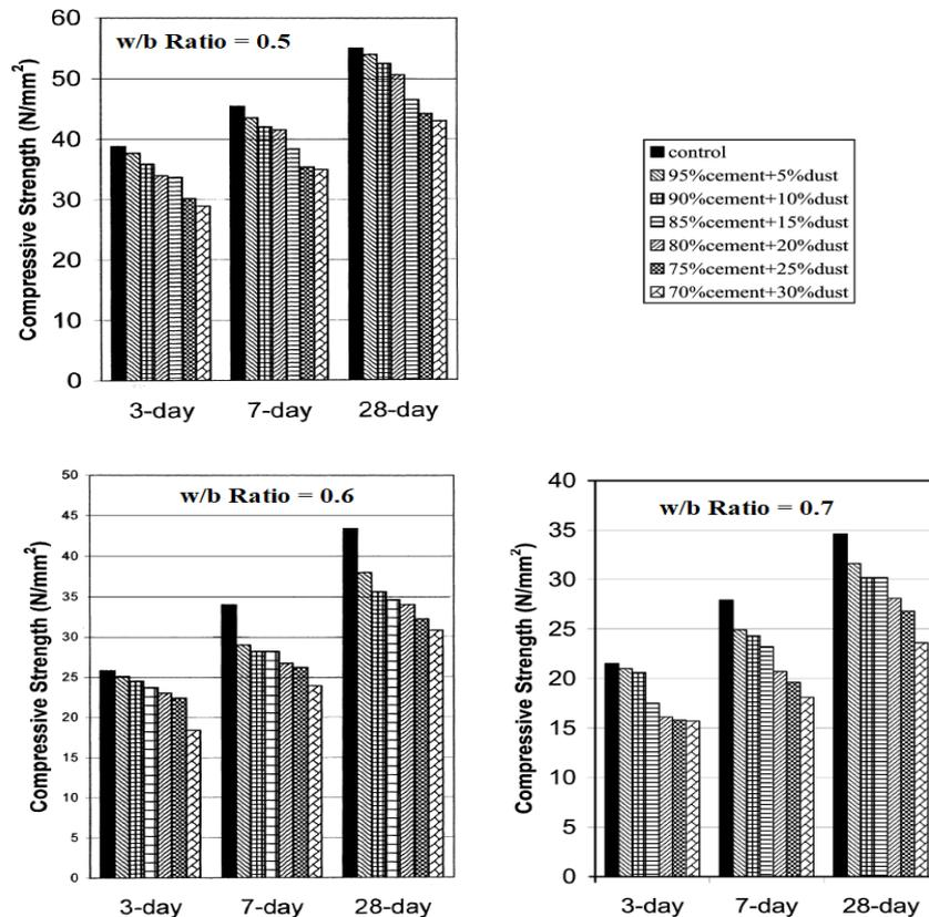
Figure 2. Effect of different w/b ratios on different concrete mix incorporation CKD [9].
