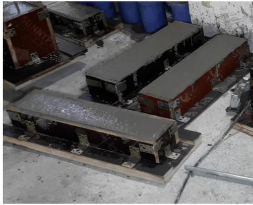
**Figure 9. Casting Concrete by Using a Beam Size 100 X 100 X 500 mm to Find the Modulus of Rupture.**
