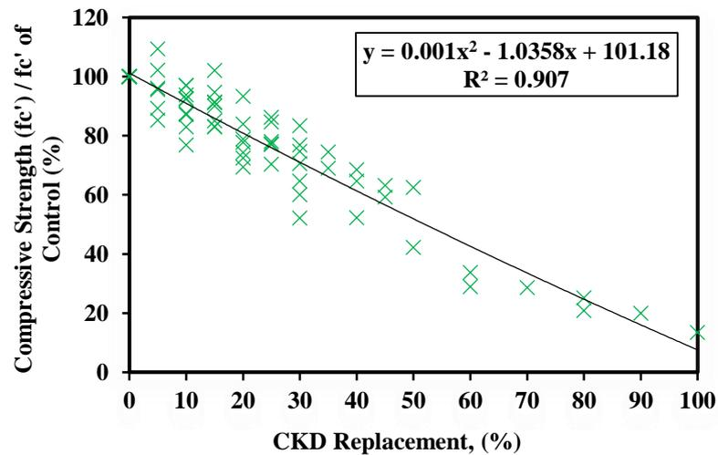
Figure 16. Non-linear Regression Model of Compressive Strength at Age 7 Days.
