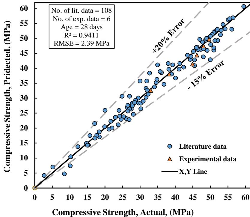
Figure 20. Relation Between the Measured and Predict Compressive Strength at 28 Days.
