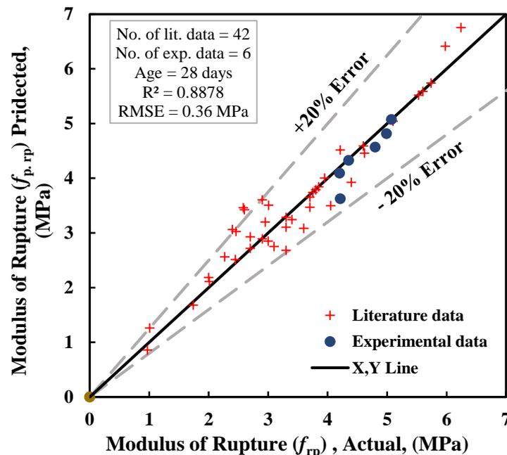
**Figure 23. Relation Between the Measured and Predict Flexural Strength at 28 Days.**
