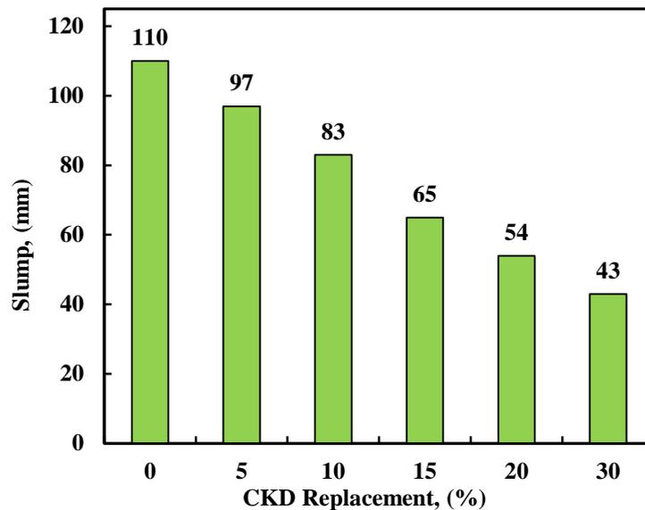
**Figure 11. Effect of CKD on the Slump of the Concrete.**
