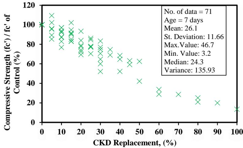
Figure 15. Statical Analysis of Compressive Strength for 7 Days, Collected from Table 1.
