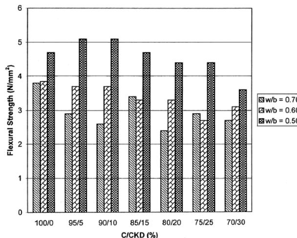
Figure 5. Effect of CKD on flexural strength of concrete [9].
