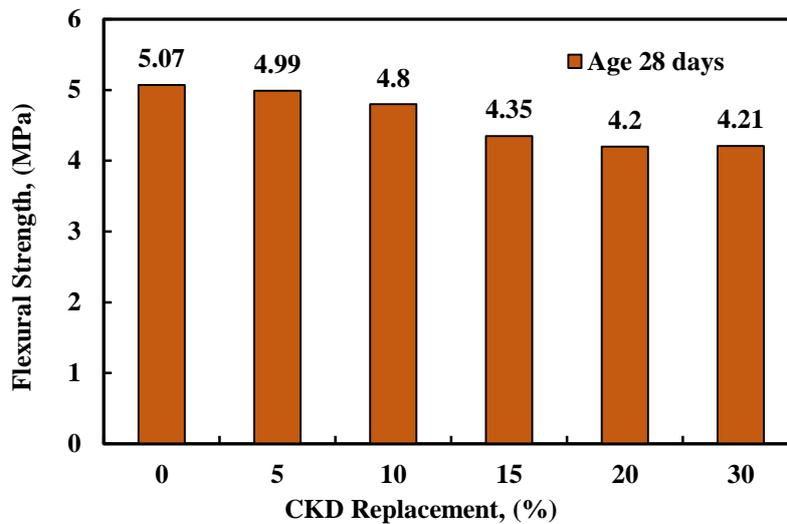
**Figure 14. Effect of CKD on the Flexural Strength of the Concrete.**
