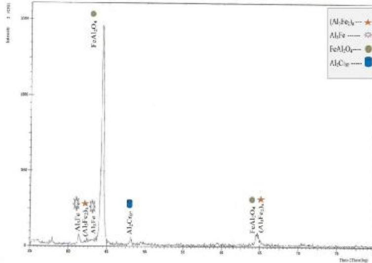
chart (c) {XRD chart for samples treated by Aluminizing +Laser }.
