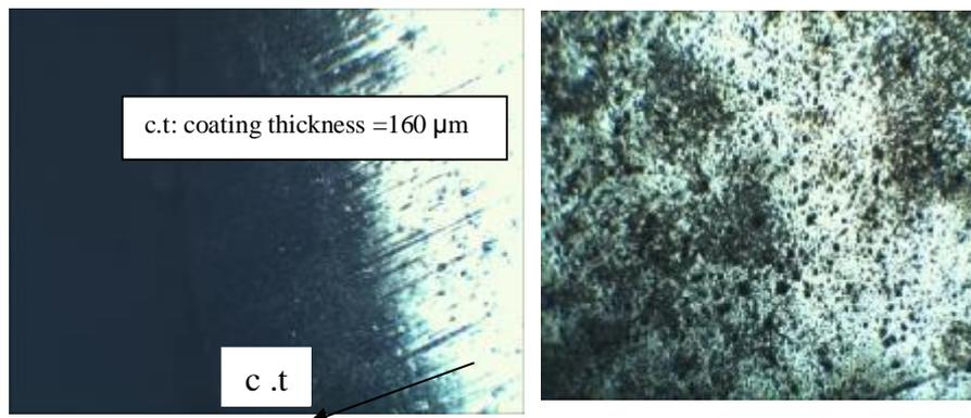
Figure (1) Image (c<sub>1</sub>) surface micro structure X 200      Figure (1) Image (c<sub>2</sub>) core of diffusion coated systems X 200
