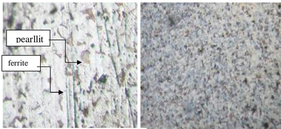
**Figure (1) Image (a<sub>1</sub>) microstructure for as received condition X200**
