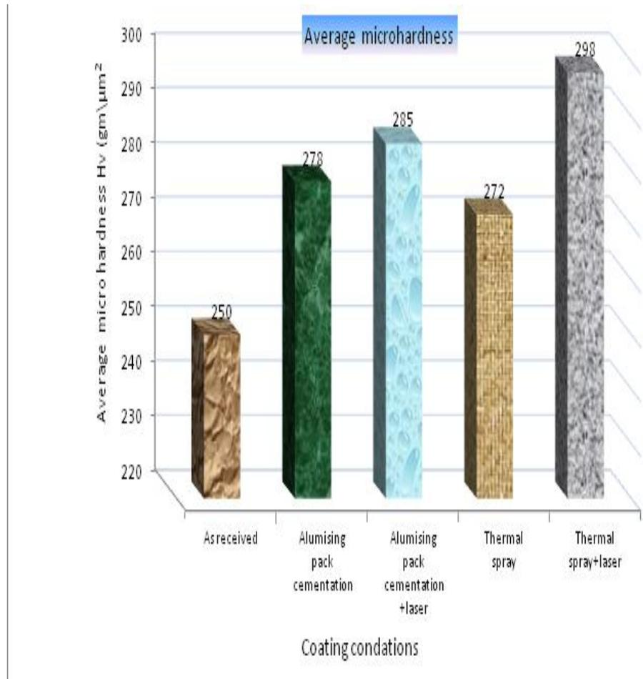
**Figure (4b) A histogram showing the behavior of average micro hardness for (200 $\mu$ m) to all the selected treatments and for the laser treated surface coated systems.**
