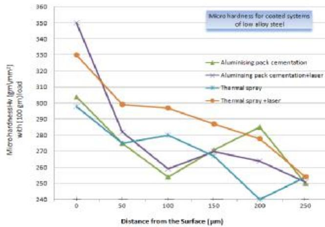
Figure (3) Micro hardness profiles curves of, (diffusion coated (aluminizing), thermal spray coated systems and for the laser treated surface coated systems.
