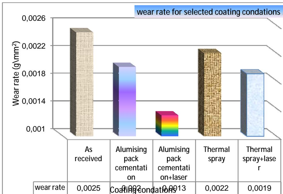
Figure (4a) A histogram diagram illustrating surface treatment influence on a wear rate of low alloy steel treated with surface treatment and laser surface treatment.
