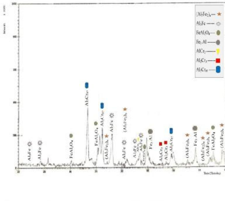
Chart (d) {XRD chart for samples treated by Thermal Spray +Laser}
