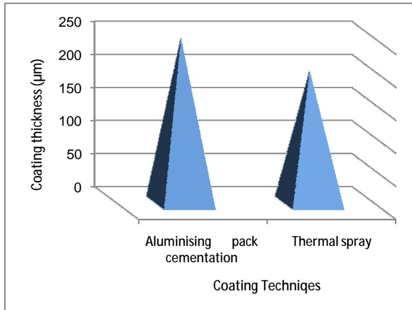
Figure (5) Rough estimated Coating thicknesses (µm) for Coating techniques.
