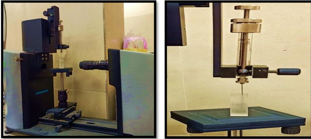
Figure 4. (A) present the tensiometer apparatus. (B) When the interfacial tension is measured.
