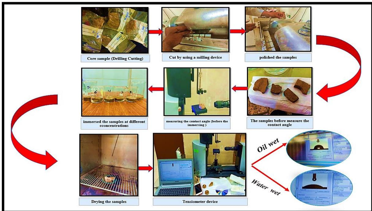
Figure 3. Shows the steps for measuring the contact angles.
