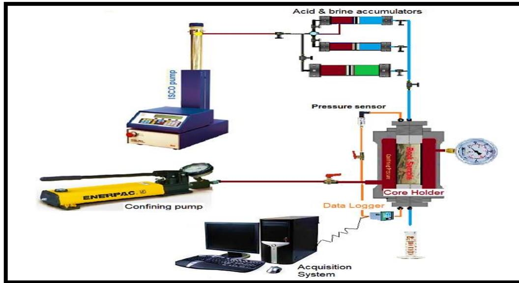
Figure 5. Schematic of the core flooding apparatus [10] [12].
