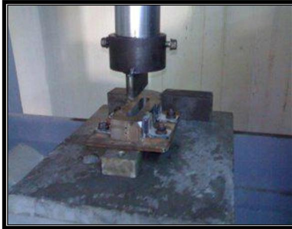
Figure (2) the punch and die used in squeeze casting
