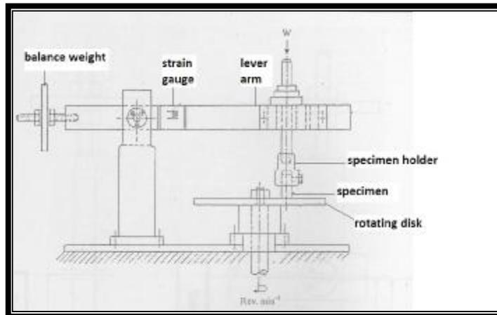
Figure (3) Wear test apparatus
