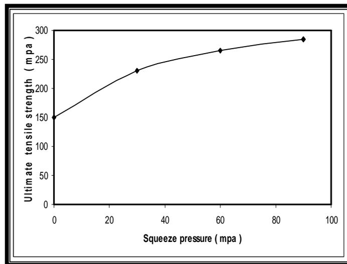
Figure (11). Effect of squeeze pressure on ultimate tensile strength
