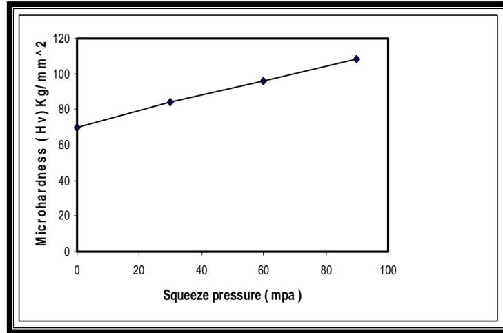
Figure (12) Effect of squeeze pressure on microhardness
