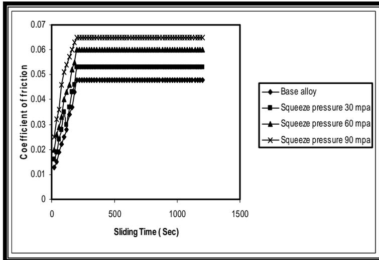
Figure (10) Coefficient of friction for the base alloy and composites which casts under different squeeze pressure in function of sliding time. Load 10 N, sliding speed 2.7 m/sec.
