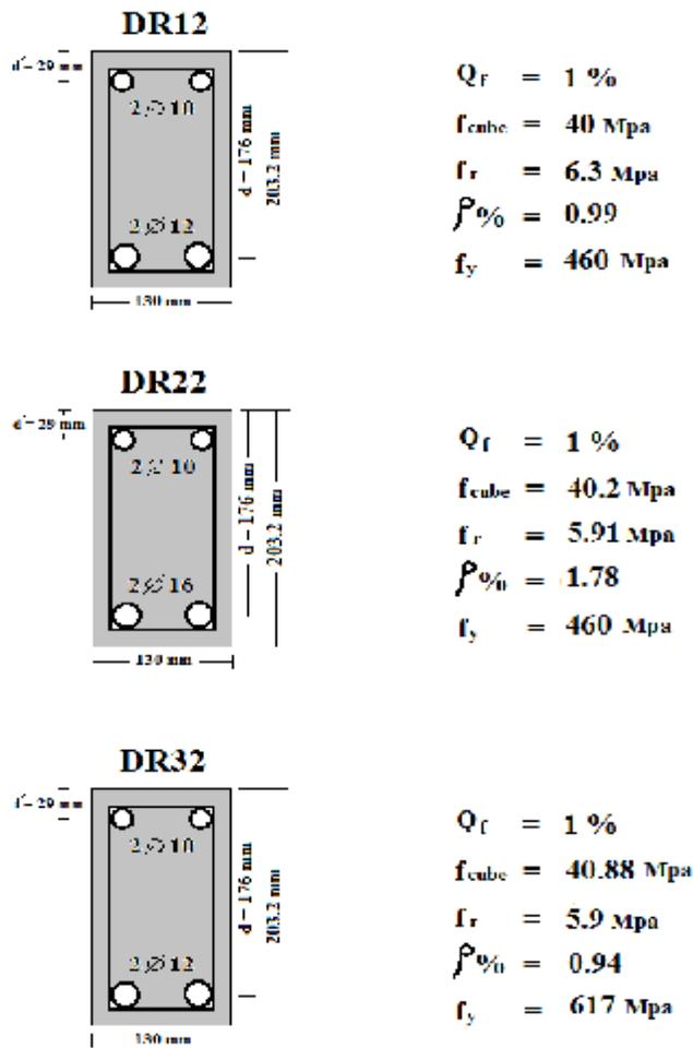
Figure (7): Details of the reinforcement and cross section of beams
