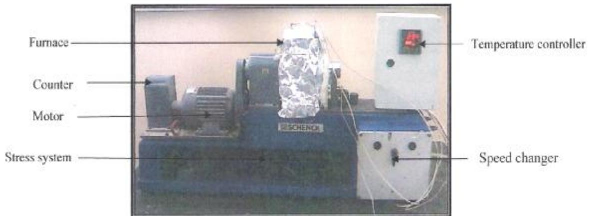
Figure (1): PUNN Rotary fatigue bending machine
