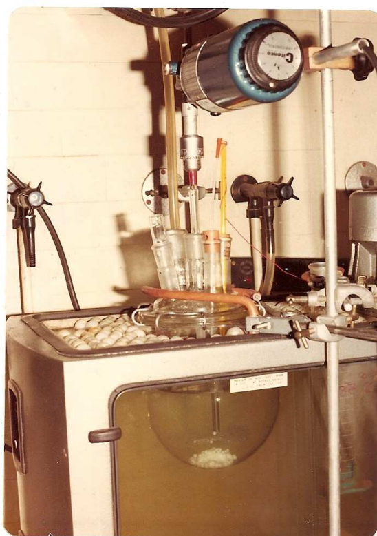
Fig. (1): Flask-stirrer apparatus used for the dissolution studies on different nitrofurantoin suspensions
