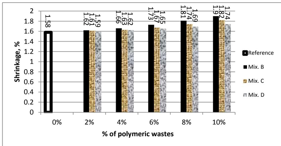
Figure 1: Effect of Polymeric Wastes on the Firing Shrinkage
