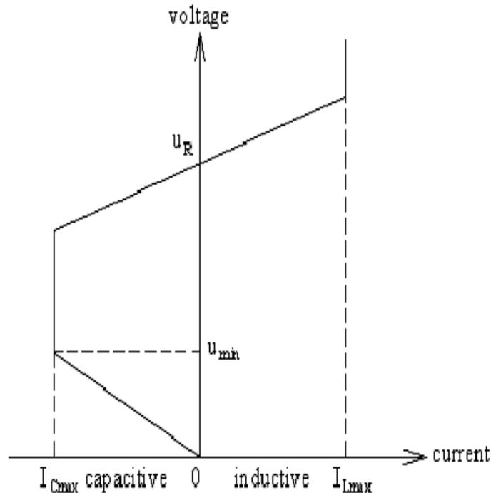
**Figure (3) voltage current characteristic of the STATCOM**
