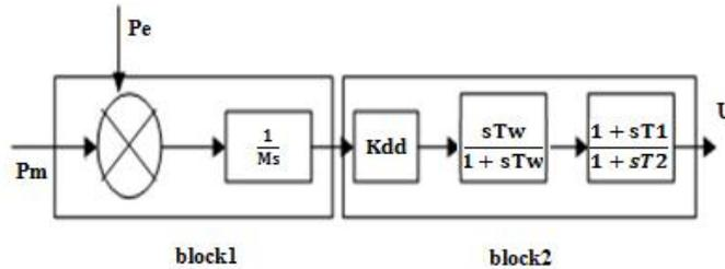
Figure (4) Transfer function block diagram of the POD
