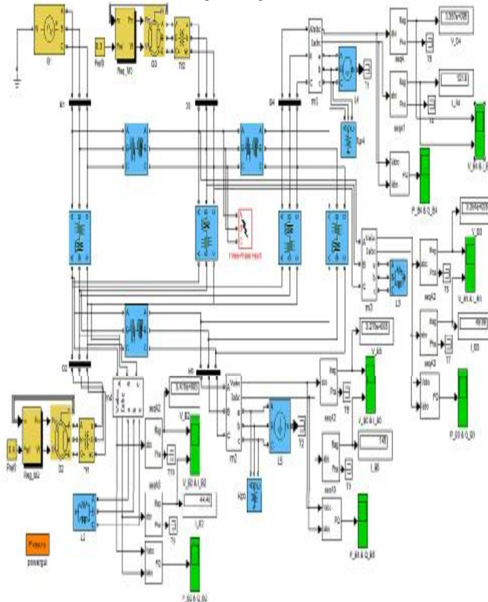
Figure (8) three phase to ground fault occur between buses (3&4)
