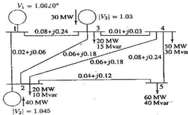
Figure (5) electrical network prototype
