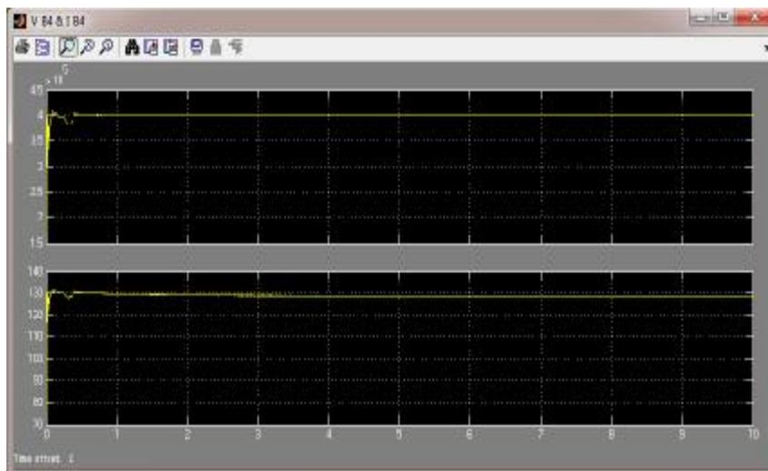
Figure (13) voltage and current on bus (4) with STATCOM
