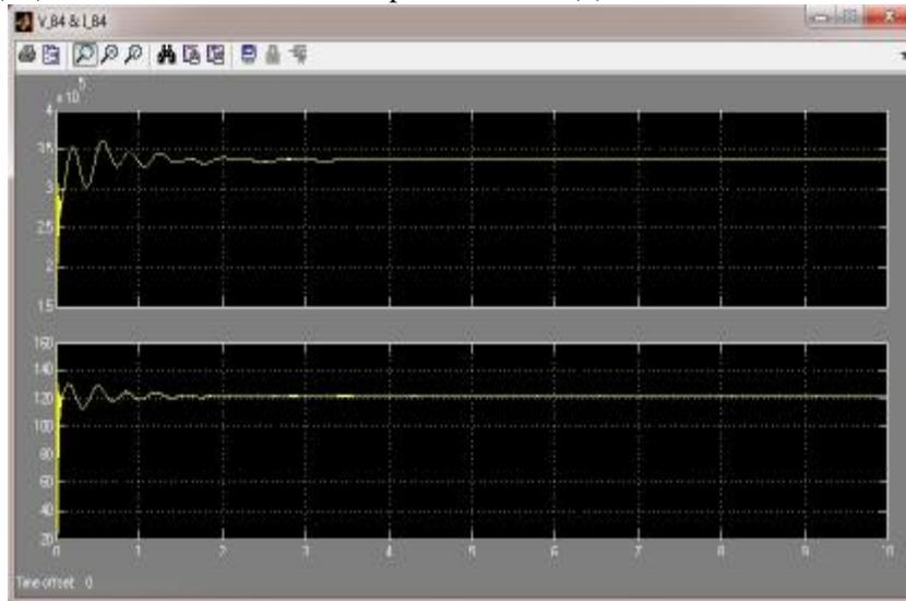
**Figure (10) voltage and current on bus (4) without STATCOM**
