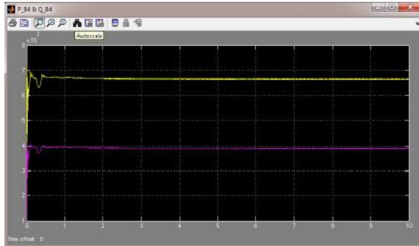
Figure (14) power and reactive power on bus (4) with STATCOM
