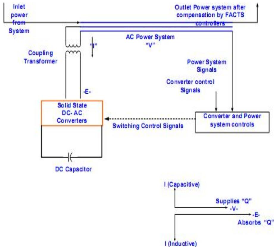
**Figure (1) Typical STATCOM compensator**
