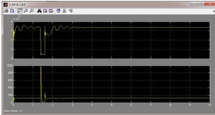
Figure (16) Voltage and current on bus (4) when fault appearing and clearing without STATCOM
