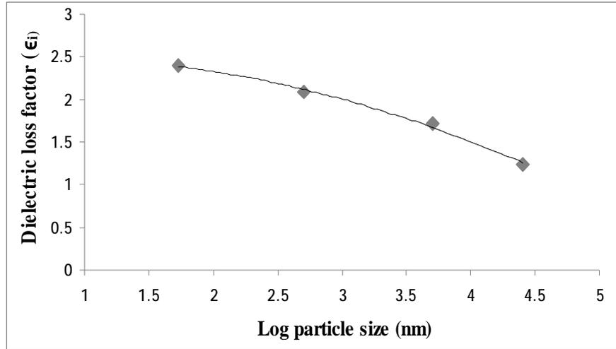
Figure (5) Dielectric loss factor against particle size of the composite at 1 MHz.
