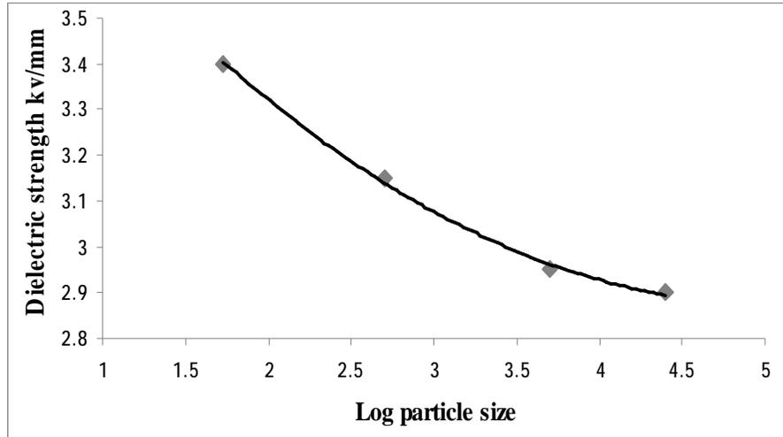
Figure (7) Dielectric strength versus particle size of the composite at 1 MHz.
