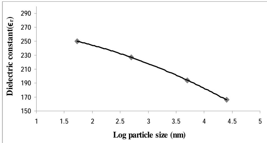
Figure (4) Dielectric constant versus particle size of the composite at 1 MHz.
