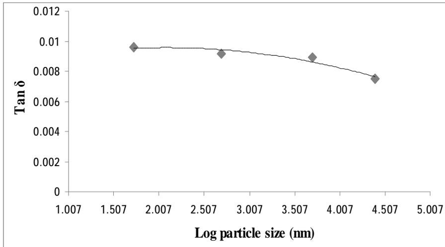
Figure (6) Tangent loss ( $\tan \delta$ ) versus particle size of the composite at 1 MHz.
