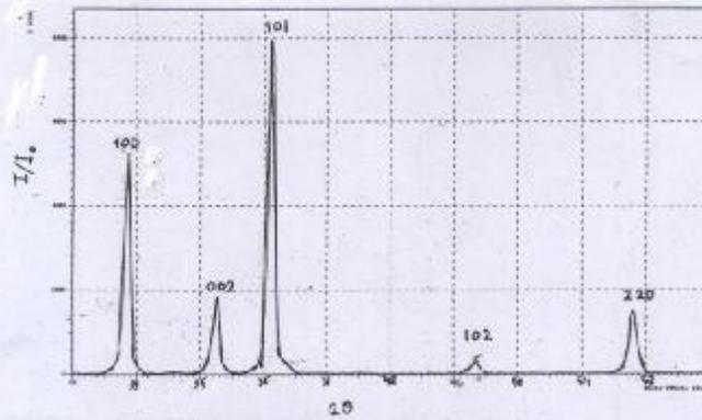
Figure(1) XRD of nanosized of ZnO powder
