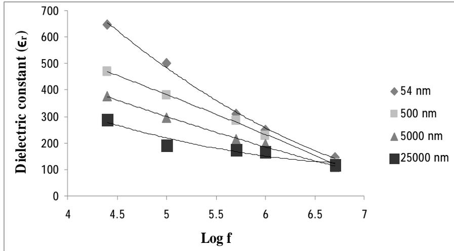
Figure (3) Dielectric constant versus frequency for the composite at different particle size.
