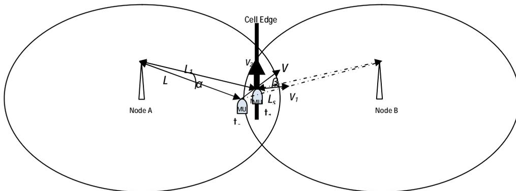
Figure (3) Schematic diagram of handover process
