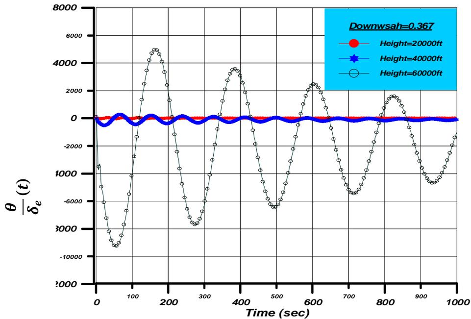
Figure (6) Variation of Height with Fixed Downwash (0.367) and Fixed Speed (600 ft/sec)
