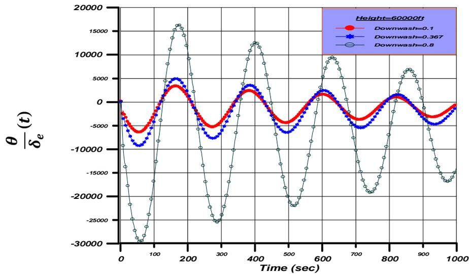
Figure (4) Variation of Downwash with Fix Height(60000ft) and Fixed Speed (600 ft/sec)
