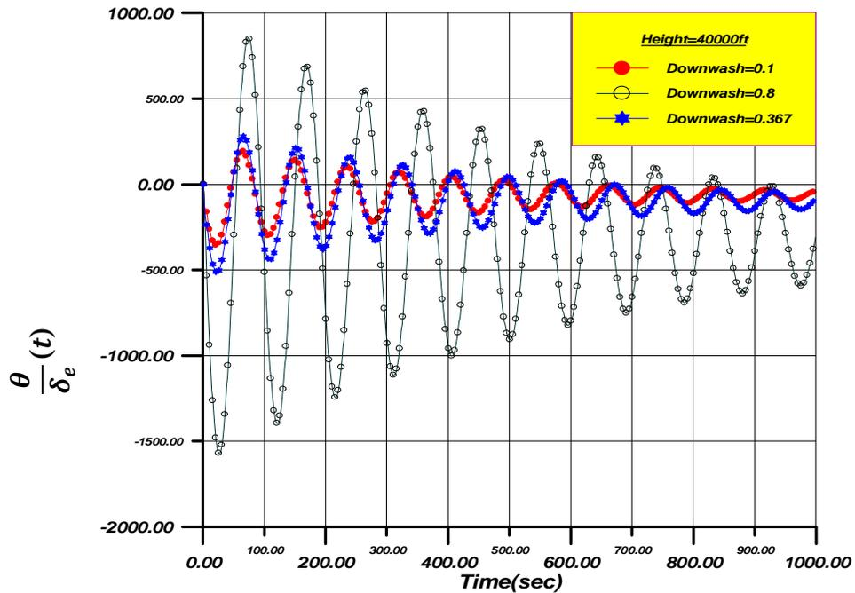
Figure (3) Variation of Downwash with Fix Height(40000ft) and Fixed Speed (600 ft/sec)
