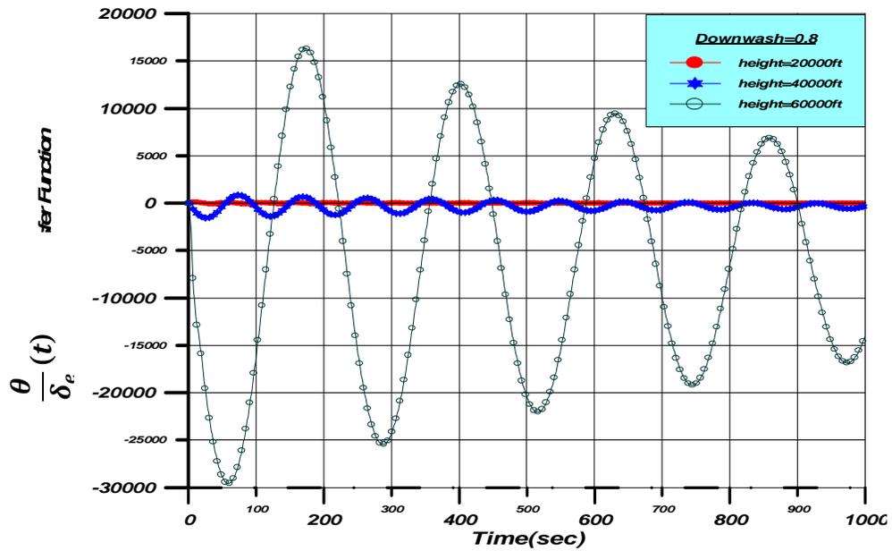
Figure (7) Variation of Height with Fixed Downwash (0.8) and Fixed Speed (600 ft/sec)
