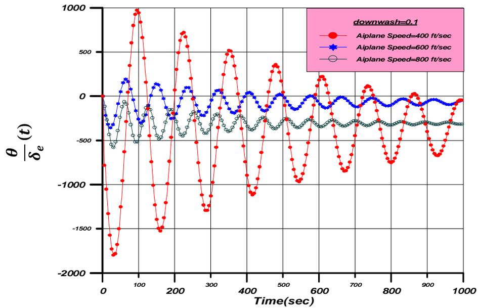
Figure(8) Variation of Speed with Fixed Downwash (0.1)and Fix Height(40000ft)
