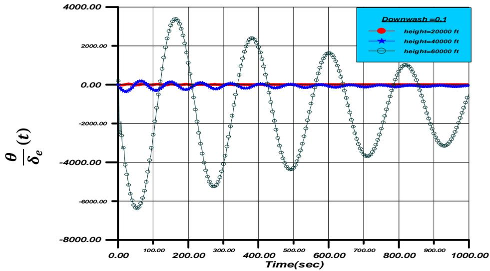
Figure (5) Variation of Height with Fixed Downwash (0.1) and Fixed Speed (600 ft/sec)
