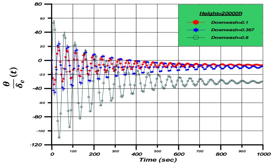
Figure (2) Variation of Downwash with Fix Height(20000ft) and Fixed Speed (600 ft/sec)
