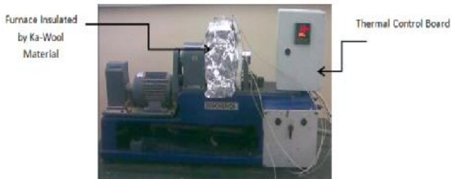
Figure (3-a) Furnace attached to the fatigue machine with the control board
