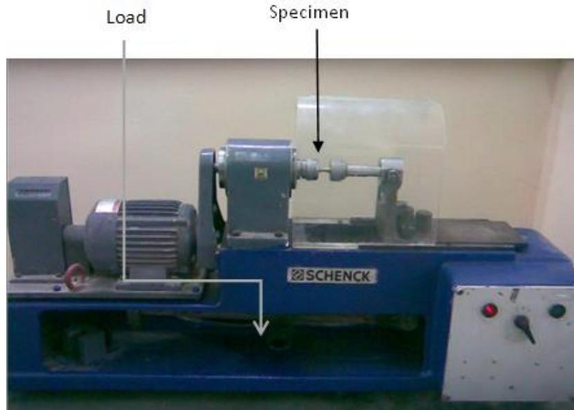
Figure (1) Machine of PUNN Rotary bending fatigue.
