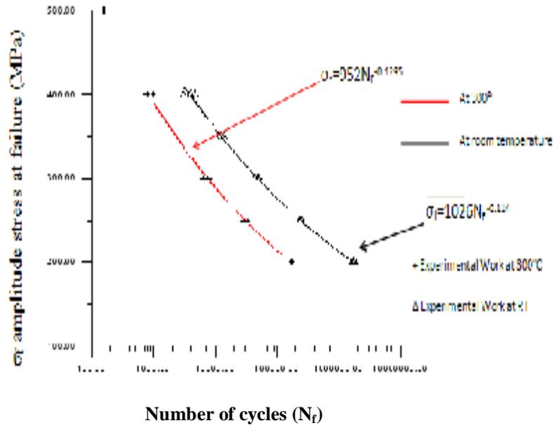
Figure (4-c) S-N curve behavior of Y10
