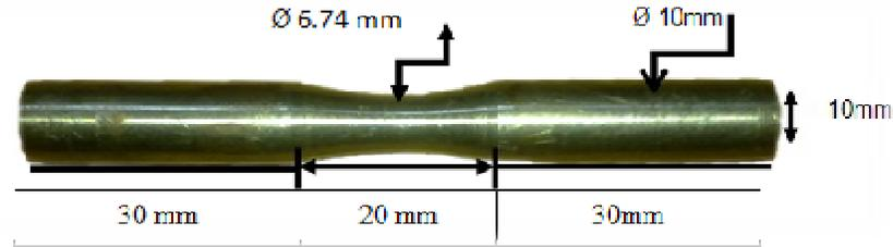
Figure (2) Fatigue test specimen according to (Din 50113) standard specification.
