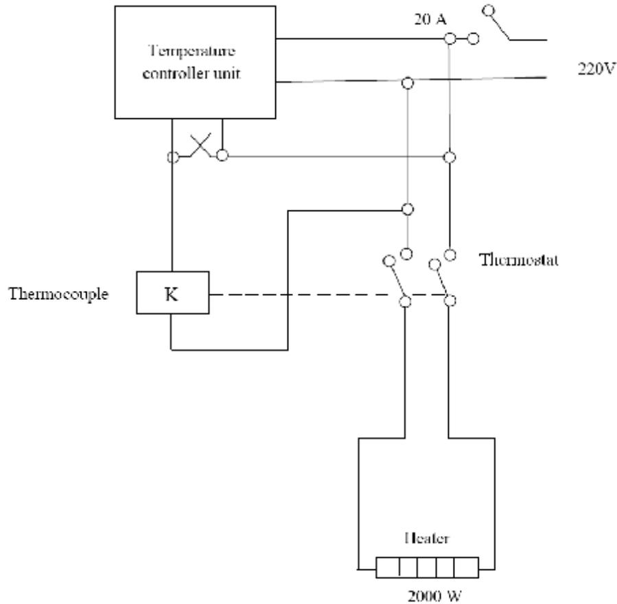
Figure (3-b) Thermal control circuit.
