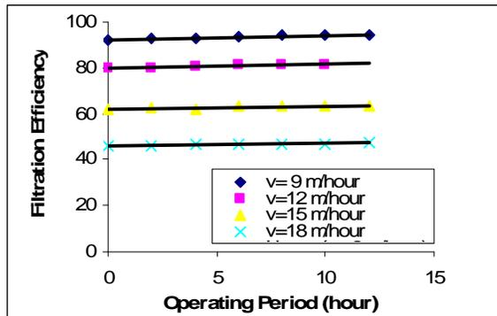
Figure (9) The Variation of Filtration Efficiency Due to Operating period for media Thickness=130 cm
