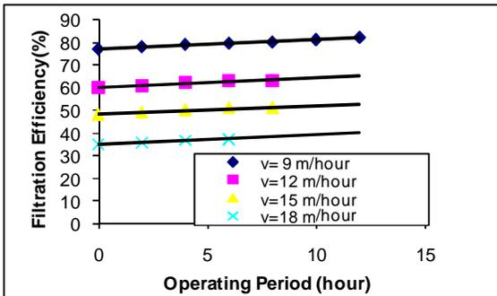
Figure.(5) The variation of filtration efficiency due to operating period for media thickness=90cm
