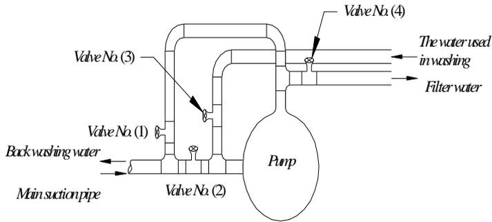
Figure (2) the Pattern of Changing in Pipe's Connection
