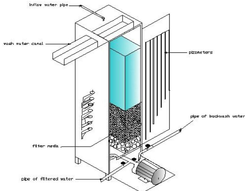
**Figure (1) Laboratory Filter**
