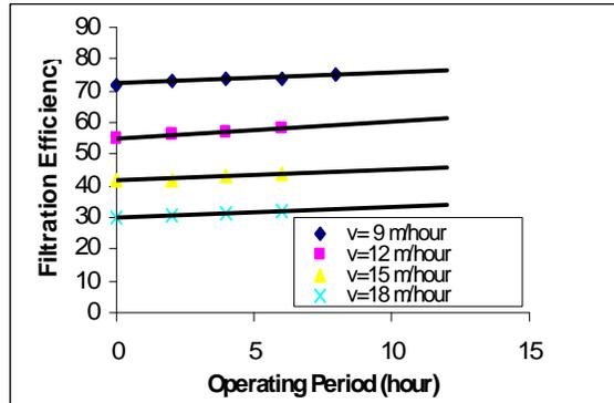
Figure (4) The variation of filtration efficiency due to operating period for media thickness=90cm
