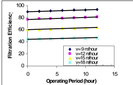
Figure.(8) The variation of filtration efficiency due to operating period for media thickness=120cm
