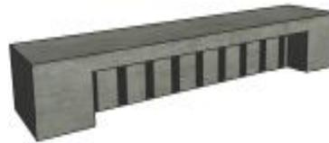
Fig (3) Strengthened Beam with 90° CFRP Strips in the Web Only (B290W)
