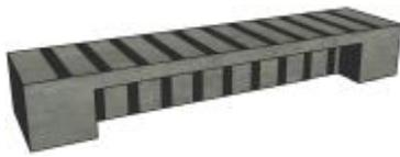
Fig (4) Strengthened Beam with 90° CFRP Strips in the Web and Flange (B390WF)
