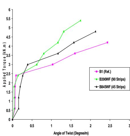
Figure (15) Torque - Twist Behavior: Effect of Fiber Orientation
