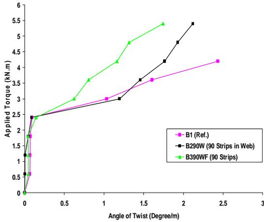
Figure (11) Torque - Twist Behavior: Effect of Flange Strengthening
