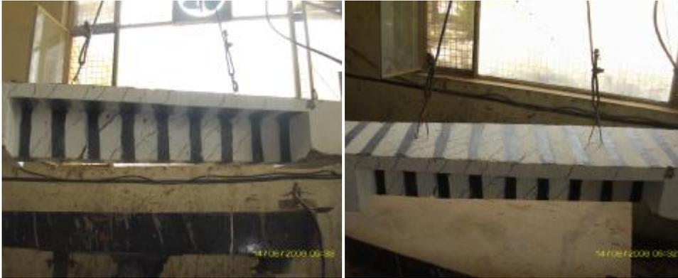
**Figure (14) Mode of Failure of Strengthened Beam
