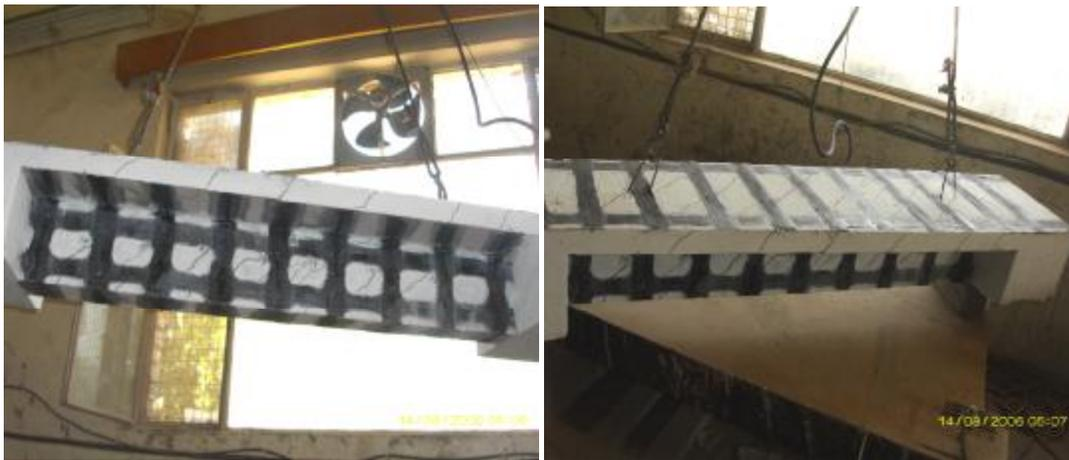
Figure (20) Mode of Failure of Strengthened Beam B690WFL (90° Strips + Long. Strips)
