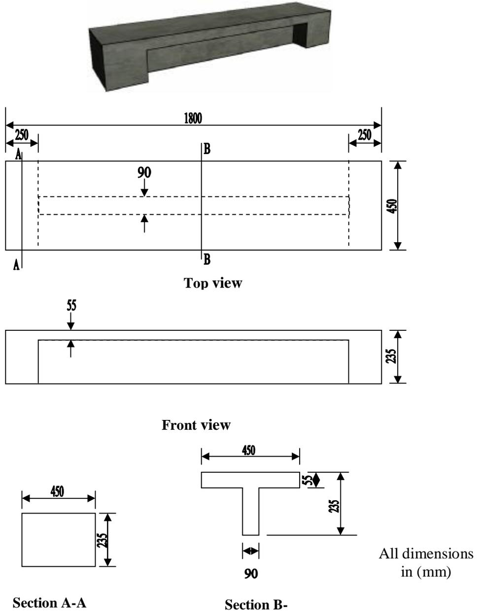
Figure (1) Beam Specimen with Dimensions
