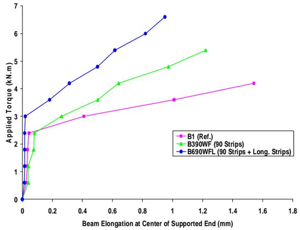
Figure (19) Beam Longitudinal Elongation Behavior: Effect of Strengthening in Longitudinal and 90° Transverse Direction
