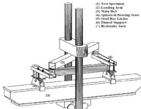
Figure (9b) Schematic Diagram Testing
