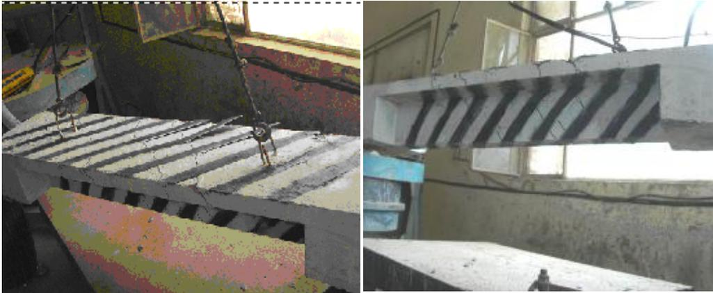
**Figure (17) Mode of Failure of Strengthened Beam B845WF (45° Strips in Web and Flange)**
