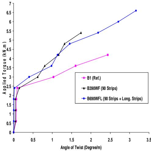
Figure (18) Torque - Twist Behavior: Effect of Strengthening in Longitudinal and 90° Transverse Direction
