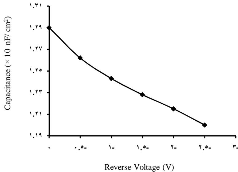
**Figure (8) The variation of capacitance versus reverse bias voltage for CdSe/Si heterojunction**
