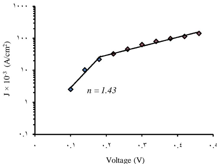
Figure (5) forward bias characteristics of a (n-CdSe/p-Si) heterojunction at room temperature.
