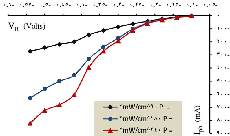
Figure (6) Reverse bias characteristics under illumination at different intensity level .
