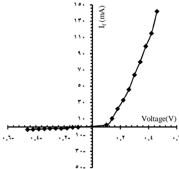
**Figure (4) Current-voltage characteristics for N-CdSe/p-Si heterojunction**
