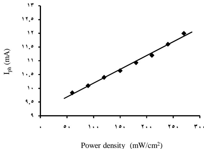
Figure (7) Photo current versus incident power density for n-CdSe/p-Si junction
