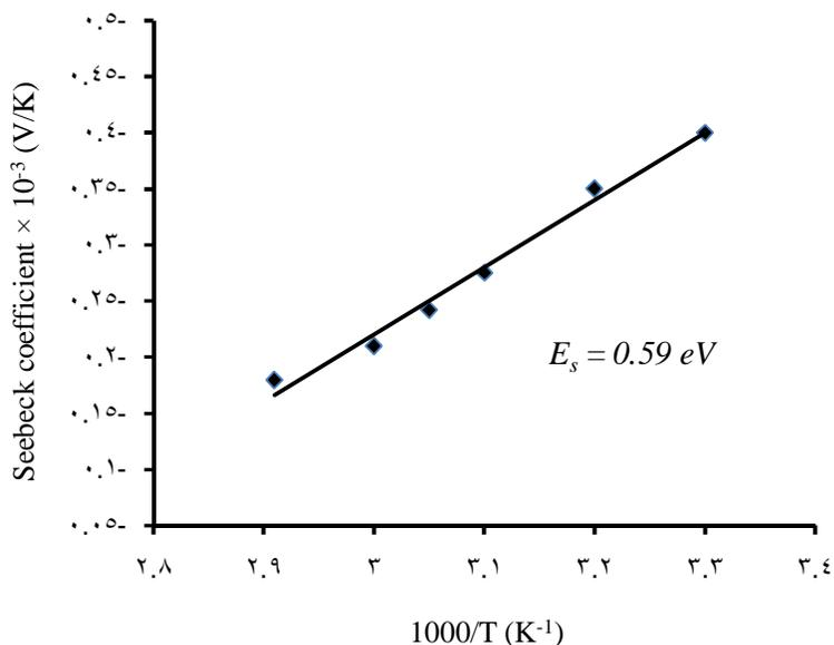
Figure (3) Temperature dependence of Seebeck coefficient For CdSe thin film.
