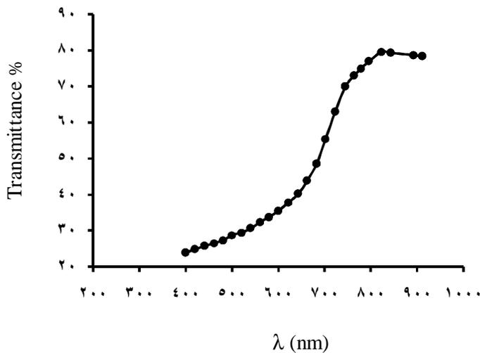
Figure (1) Transmittance spectrum of CdSe thin film
