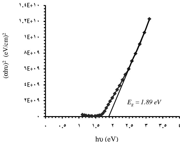
Figure (2)  $(\alpha h\nu)^2$  versus  $h\nu$  plot of CdSe thin film.
