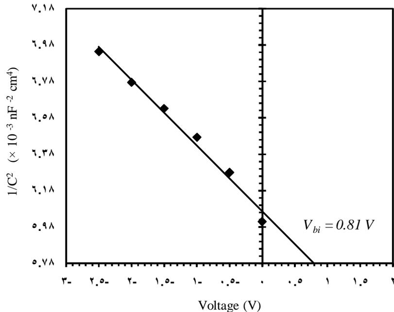
Figure (9)  $1/C^2$  vs  $V_R$  for n-CdSe/p-Si heterojunction.
