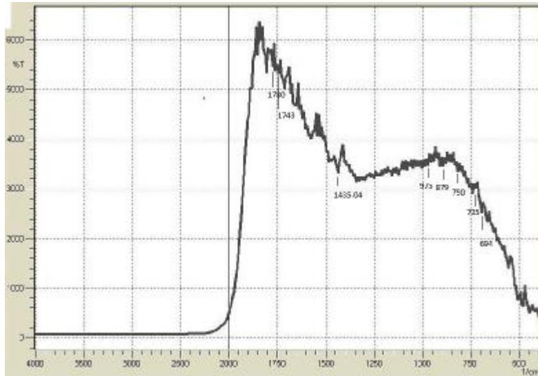
Figure (2): FTIR peaks of oxidized SnO<sub>2</sub> films at 40 minutes.
