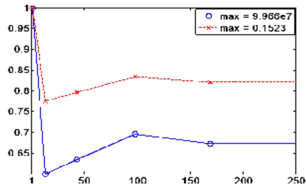
**Figure (4) Normalized I<sub>max</sub> (dotted line) and AF (solid line) as a function of number of hexagons.**
