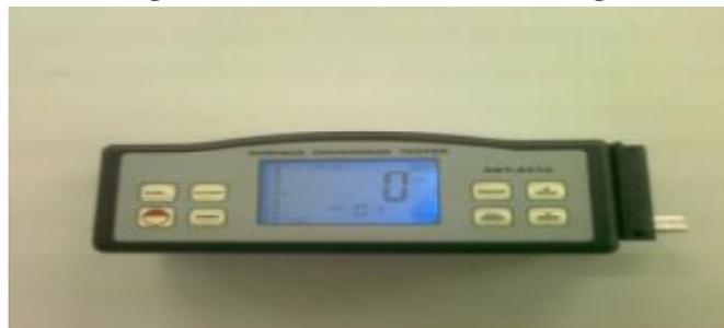
Figure (3) Surface roughness device
