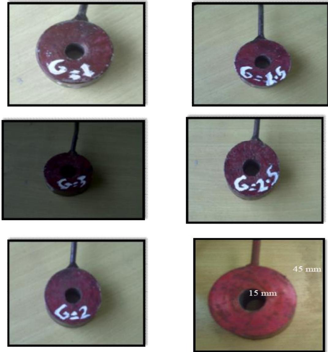
**Figure (7) The samples that used to study the effect of the gap sizes on the surface roughness and MRR**
