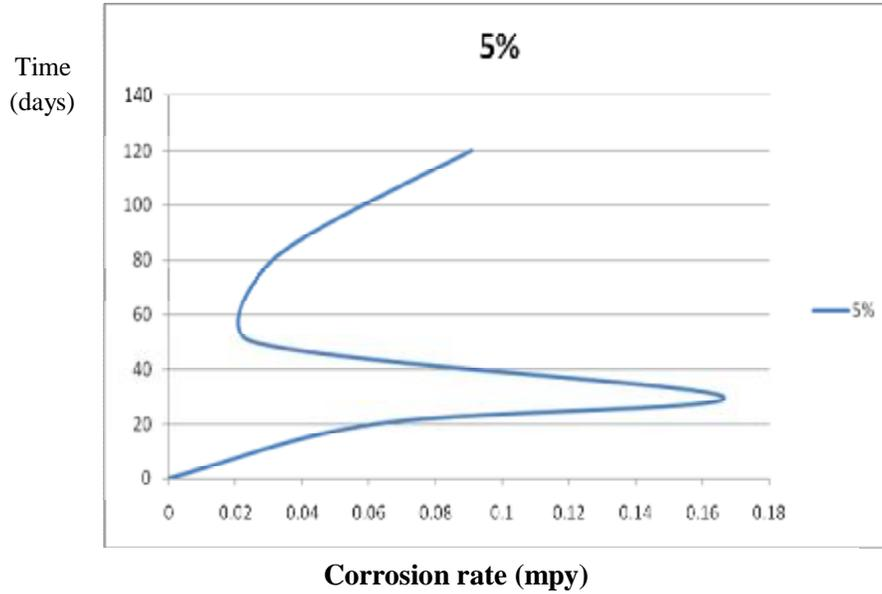
Figure (1) Relationship between corrosion rates in mpy and time in days at 5% acid concentration
