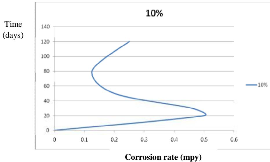
Figure (2) Relationship between Corrosion Rates in mpy and Time in Days at 10% Acid Concentration.
