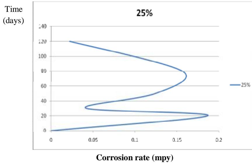
Figure (5) Relationship between Corrosion Rates in mpy and Time in Days at 25% acid Concentration.
