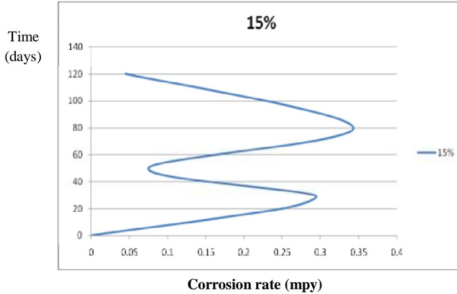
Figure (3) Relationship between Corrosion Rates in mpy and Time in Days at 15% acid Concentration.
