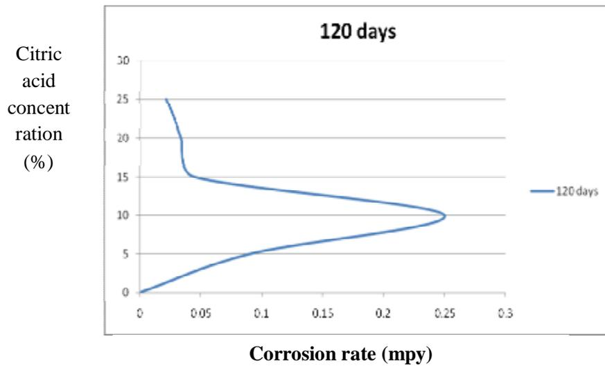
Figure (10) Relationship between Corrosion Rates in mpy and acid Concentration at 120 Days
