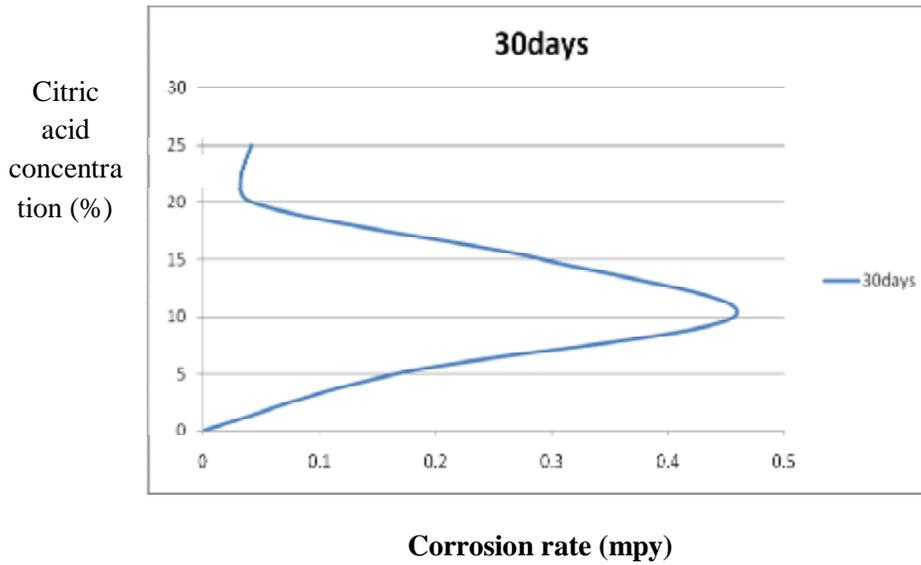
Figure (7) Relationship between Corrosion Rates in mpy and acid Concentration at 30 Days
