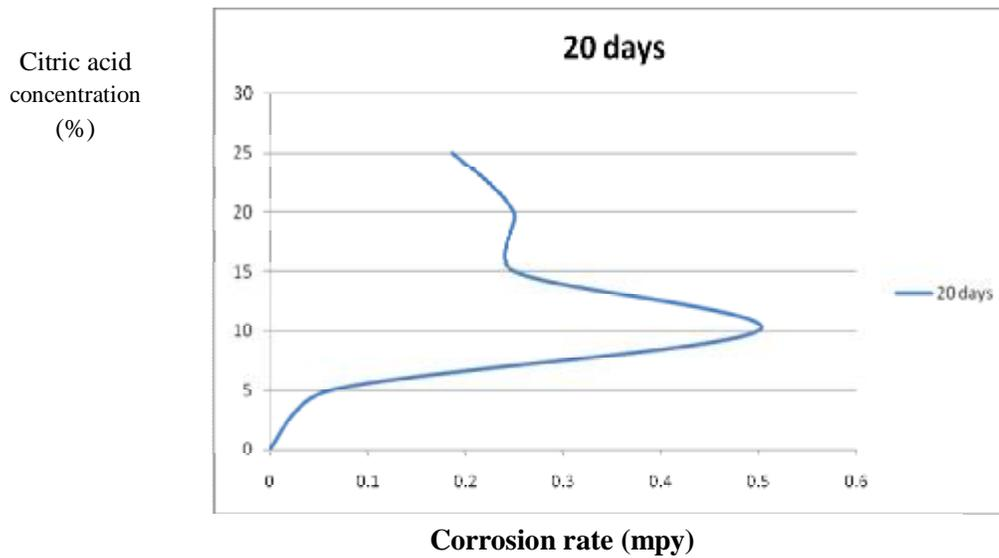
Figure (6) Relationship between Corrosion Rates in mpy and acid Concentration at 20 Days.
