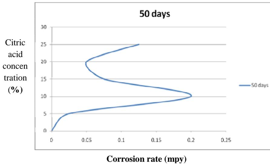
Figure (8) Corrosion Rate in mpy and acid Concentration at 50 Days
