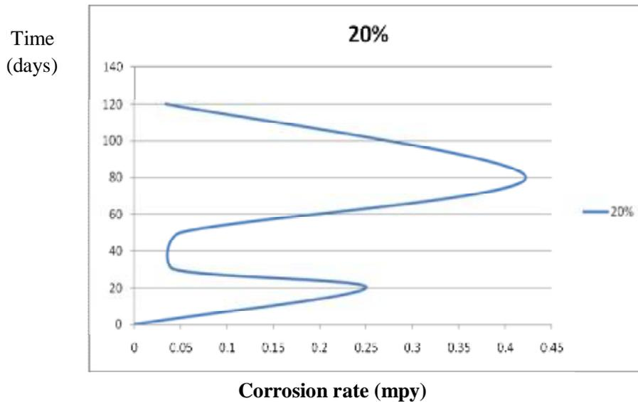
Figure (4) Relationship between Corrosion Rates in mpy and Time in Days at 20% acid Concentration.
