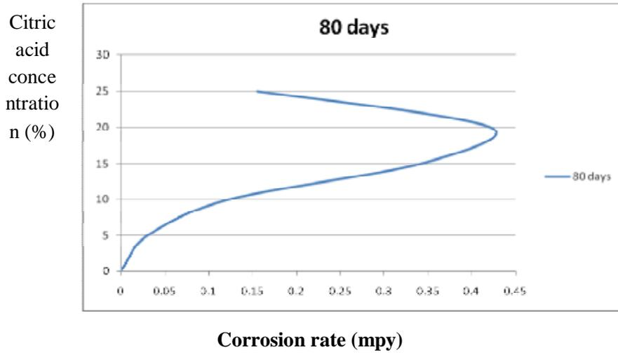
Figure (9) Relationship between Corrosion Rates in mpy and acid Concentration at 80 Days
