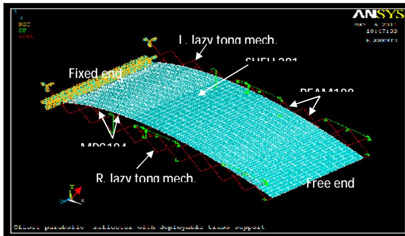
Figure (7) Loading and boundary conditions of quarter-scale of the deployable reflector.
