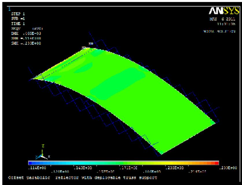
Figure (11) Von Mises stress distribution ( $N/m^2$ ) of QR scale reflector.
