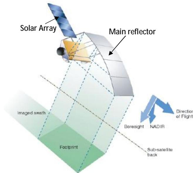
Figure (1) Traditional reflector, flight configuration.
