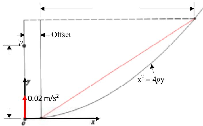
Figure (6) Profile of the reflective surface.
