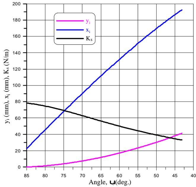
Figure ( 8) Variation of  $y_i$ ,  $x_i$ , and spring stiffness  $K_s$  through Deploying process for one pair of the truss structure.
