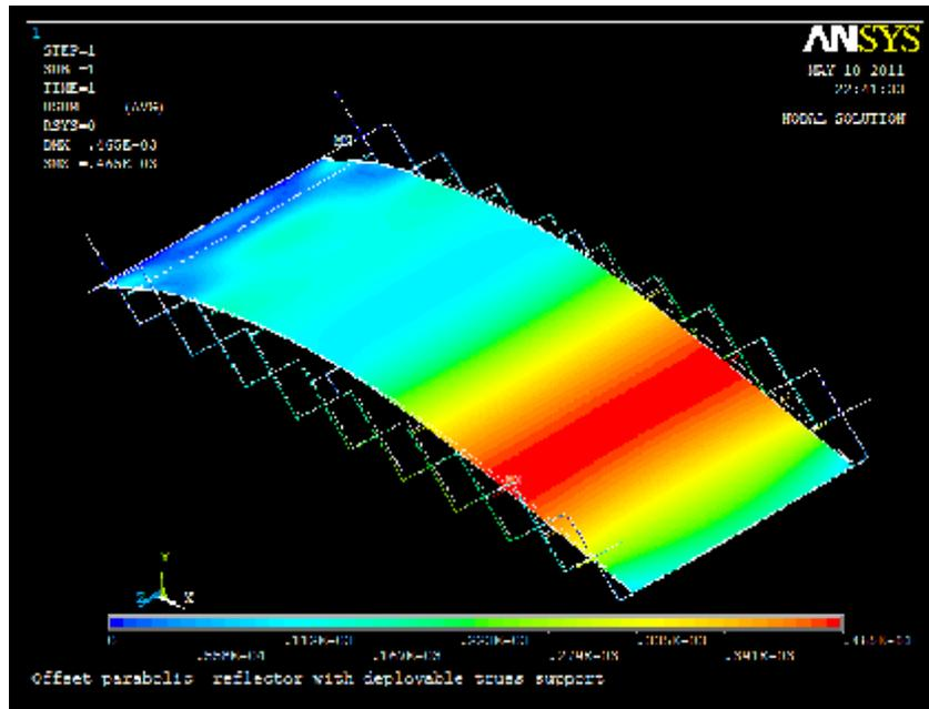
Figure (10) Distribution of maximum displacement (m) of QR scale reflector.
