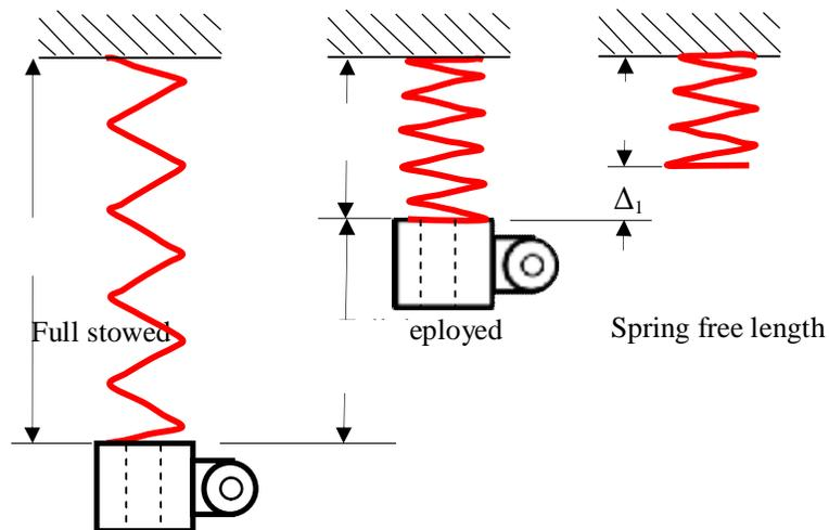
Figure (4) Length of the lower spring at fully stowed, Deployed, and free length of the spring.
