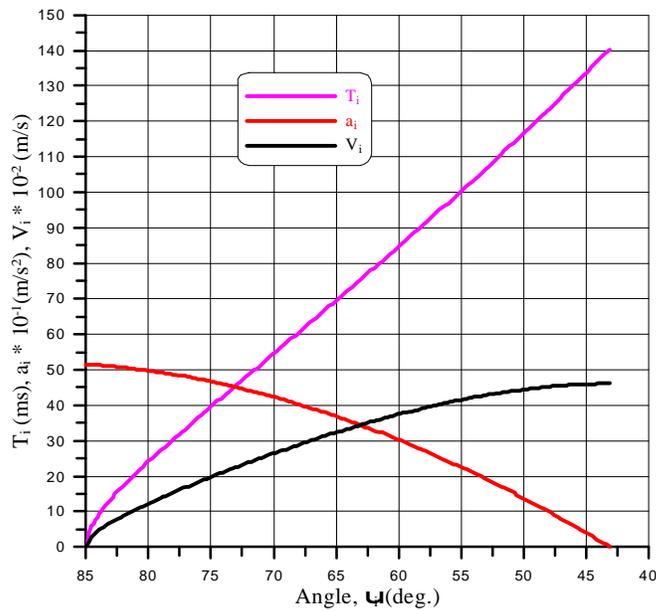
Figure (9) Time, velocity, and acceleration analysis Through deploying process.
