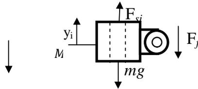
Figure (5) free body diagram of the lower moving Mass during deployment.
