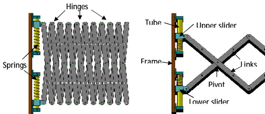
Figure (2) Solid Works representation of folding and deploying Truss (reflective surface is not shown).
