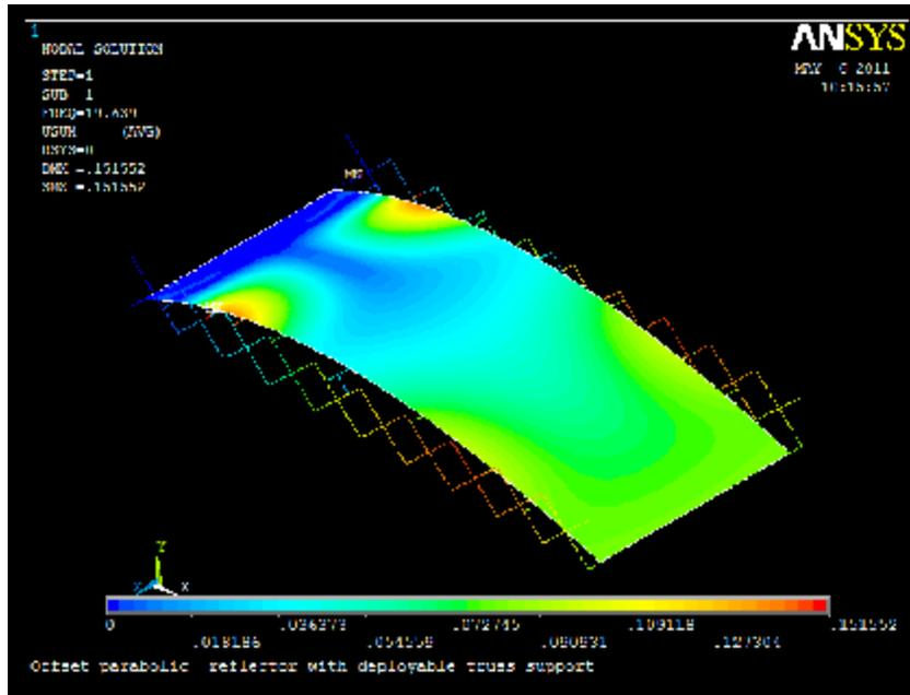
Figure (12) First mode of linear buckling (eigenvalue = 19.64) of QR scale reflector.
