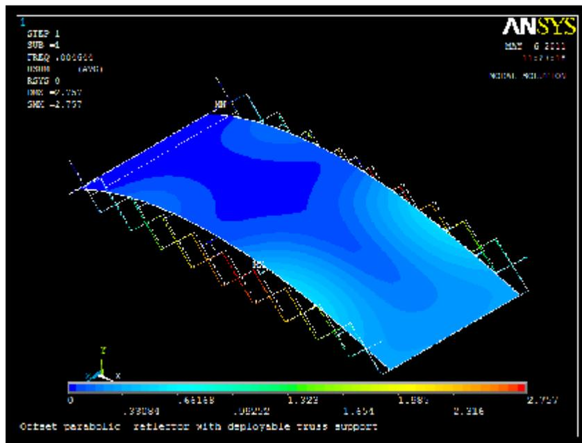
Figure (13) Fundamental natural frequency (Freq. = 0.8846 Hz) of QR scale reflector.
