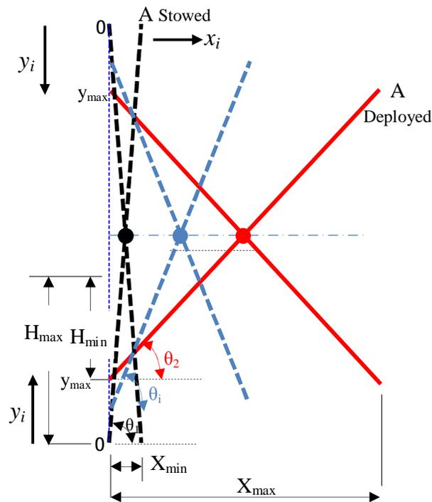
Figure (3) A sketch diagram of the stowed and deployed Configuration for one pair of the truss.
