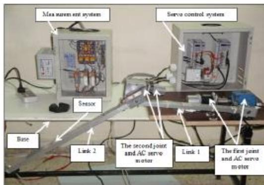
Figure (7) The semi-flexible robot for experimental work.
