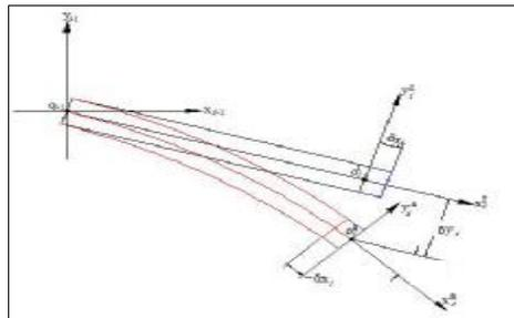
Figure (5) The coordinates system of a single semi-flexible link under deformation.
