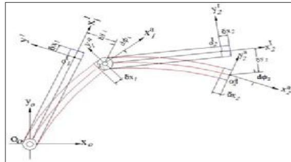
Figure (6) Coordinates systems of two links of semi-flexible robot arm.
