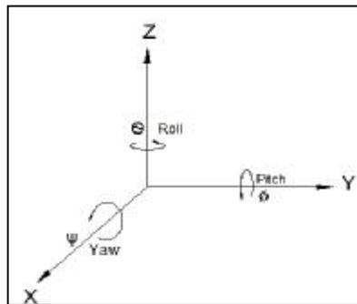
Figure (2) Roll, Pitch and Yaw coordinates for a manipulator.
