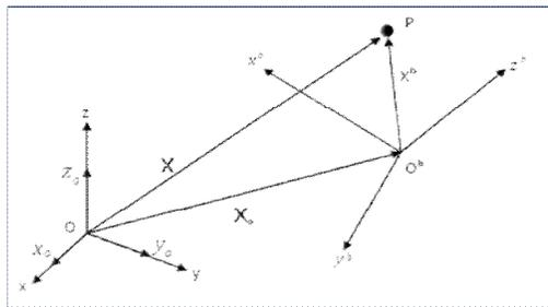
Figure (1) The position of point relative to coordinate frame.
