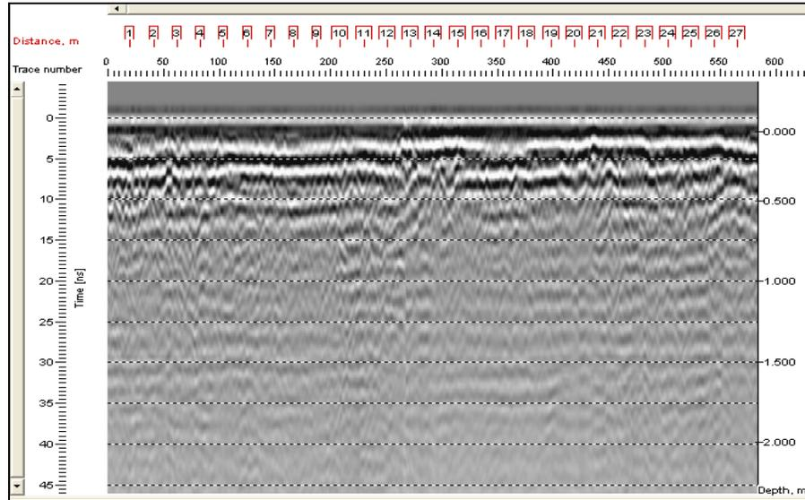
Figure (5) Reinforced bars of the roof of 1<sup>st</sup> site using 500 MHz antenna.
