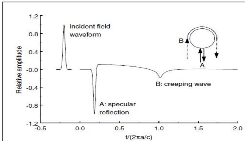
Figure ( 4) Back-scattered by a conducting sphere [8].
