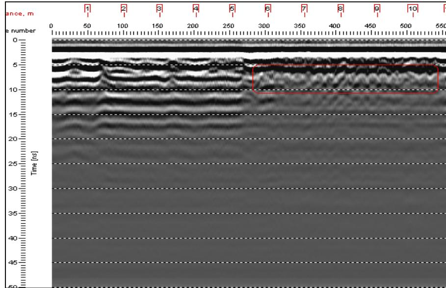
Figure (7) Reinforced bars in the foundation of the 2<sup>nd</sup> site using 500 MHz antenna.
