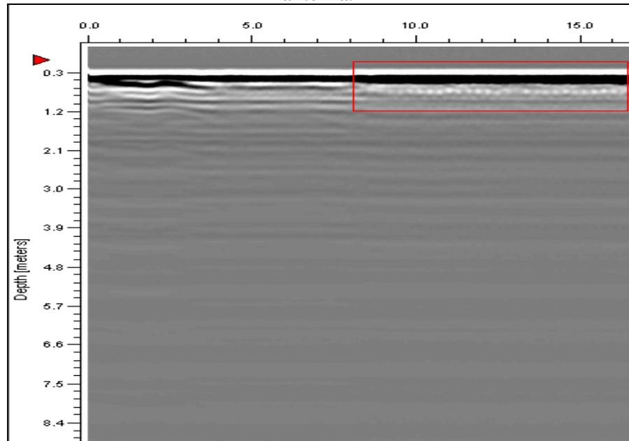
Figure (8) Reinforced bars in the foundation of the 2<sup>nd</sup> site using 250 MHz antenna.
