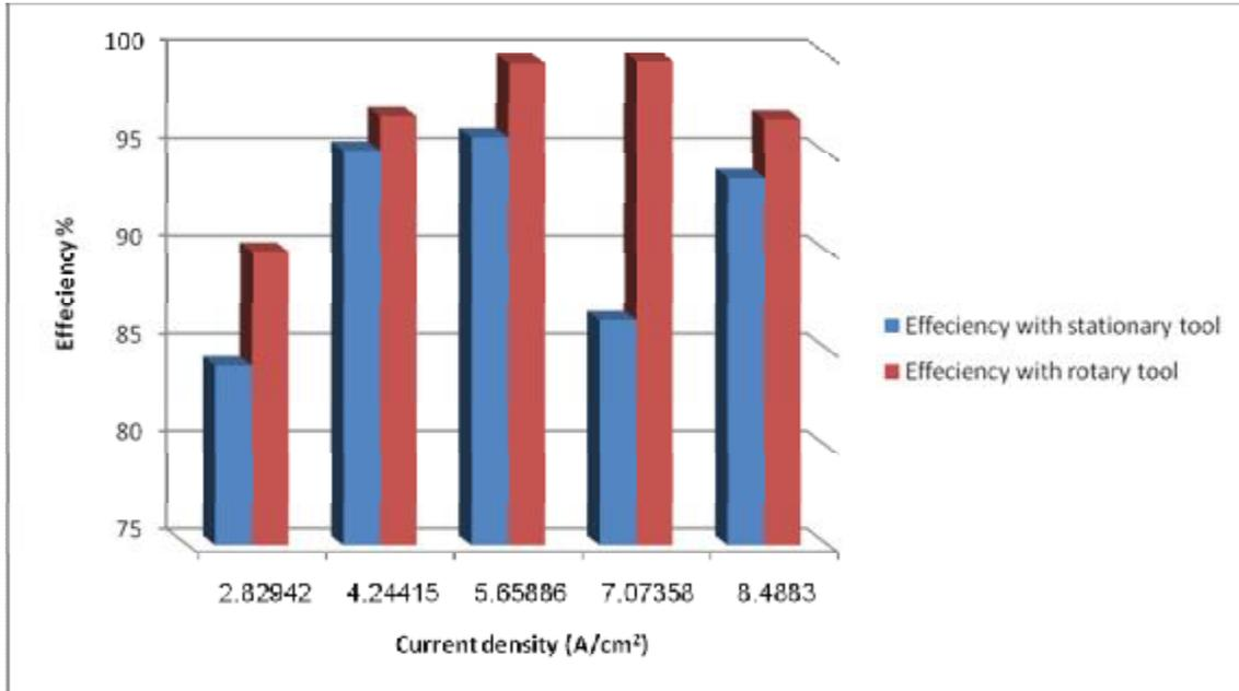
Figure (6) Efficiency of rotary and stationary tools at different current densities
