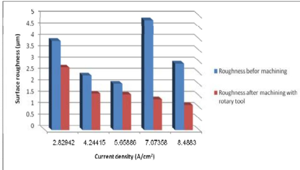
Figure (8) The differences in surface roughness before and after ECM machining in different current densities with rotational tool
