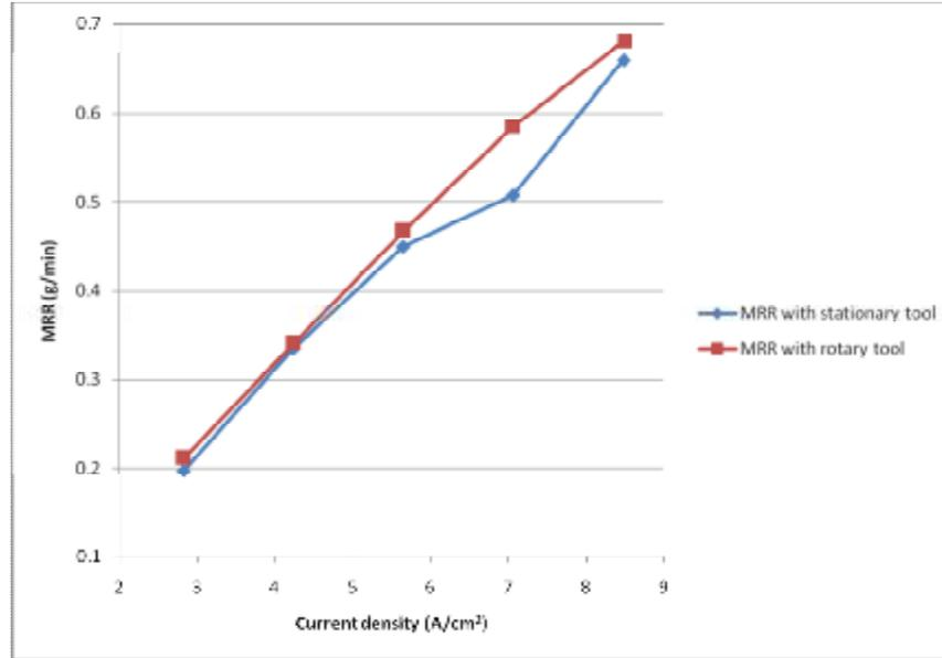
Figure (5) Experimental MRR in rotary and stationary cases
