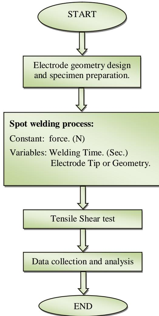
Figure (2): Flow chart illustrating the experimental procedure.
