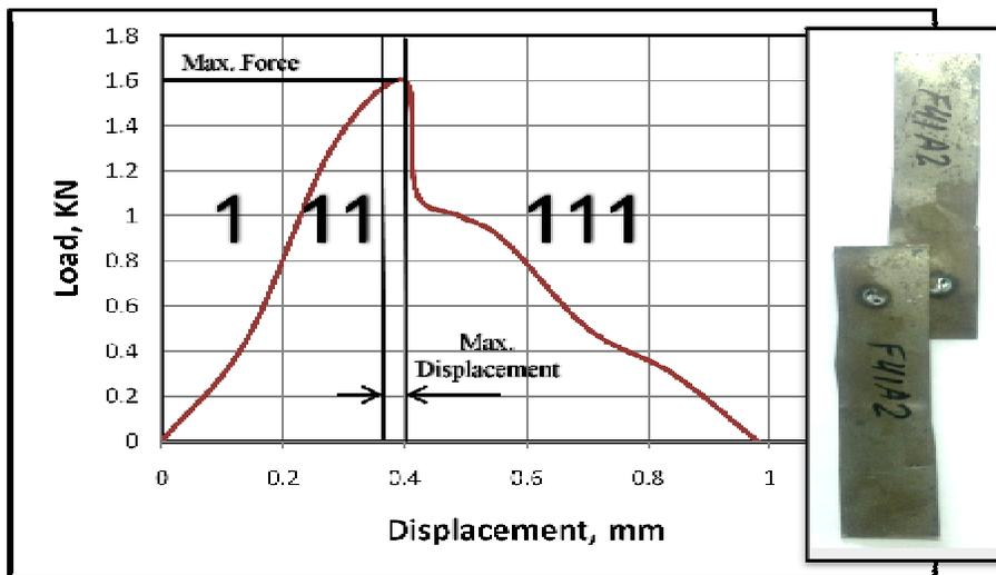
Figure (8): Represents the relationship between the displacement and force when applied tensile shear test on the welded specimen at welding variables: Punch/Flat Electrode, Time = 2 sec., constant force = 450 N.
