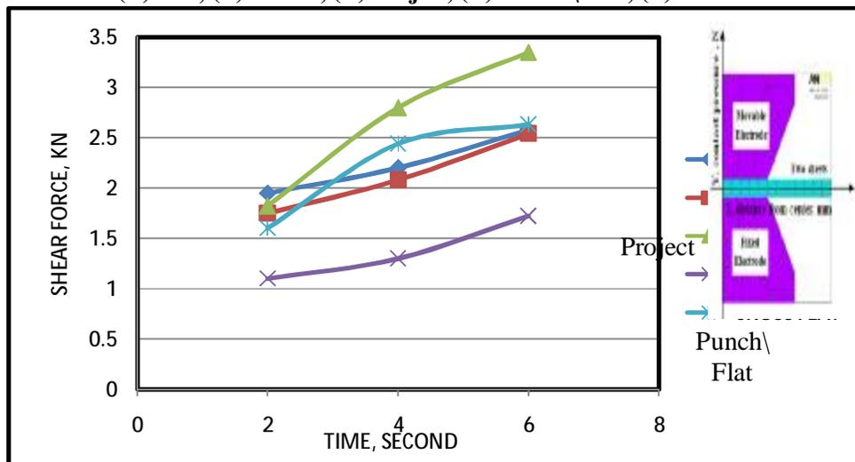
Figure (10): Represents the relationship between shear force and time practically of all specimens at Constant force = 450 N of electrode types, (A) Flat, (B) Round, (C) Project, (D) Punch / Flat, (E) Cross Flat. at constant welding Pressure = 450 N.
