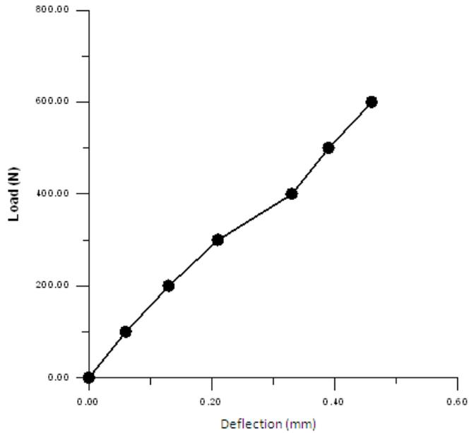
Figure (5) The load – displacement of epoxy matrix composite reinforced with 1 % wt okra fiber.
