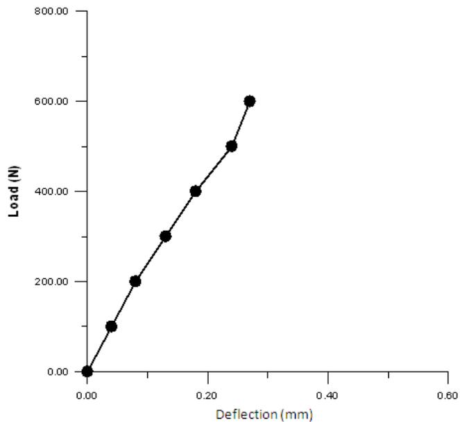
Figure (8) The load – displacement of epoxy matrix composite reinforced with 9 % wt okra fiber.
