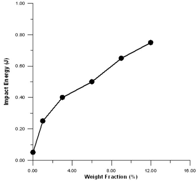
**Figure (11)Effect of weight fraction of short okra natural fiber on impact energy of epoxy matrix composite.**
