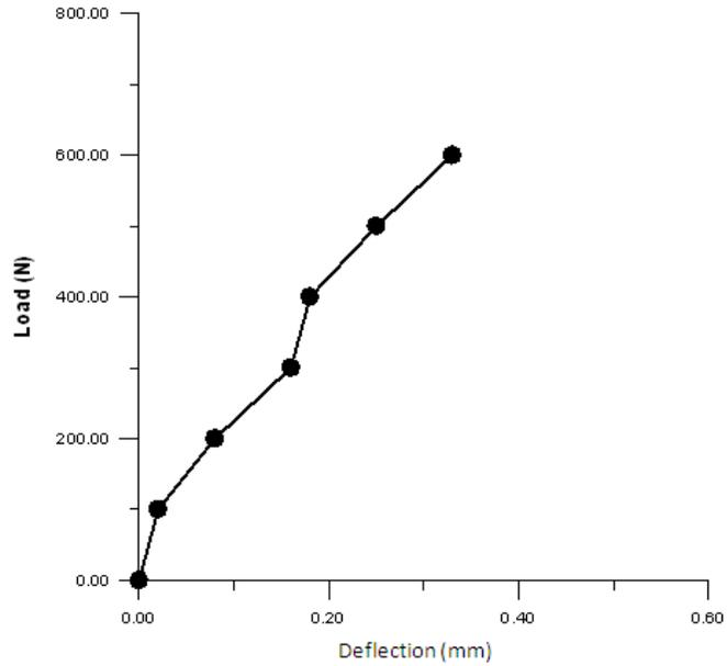
Figure (7) The load – displacement of epoxy matrix composite reinforced with 6 % wt okra fiber.
