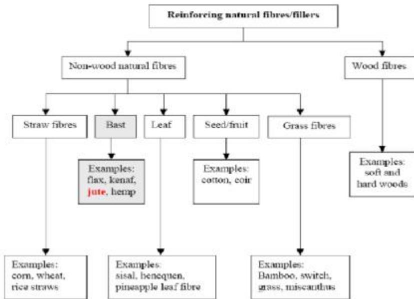
Figure (1) Classification of natural fibers which can be used as reinforcement of polymer [4].
