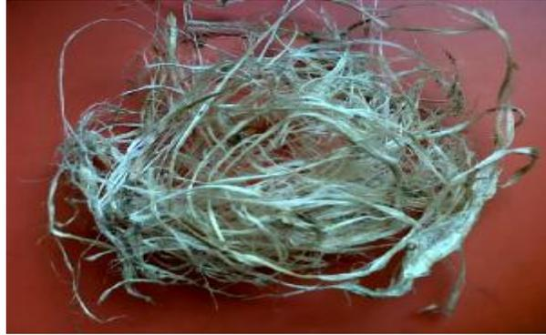
**Figure (2)**Extracted okra fibers.
