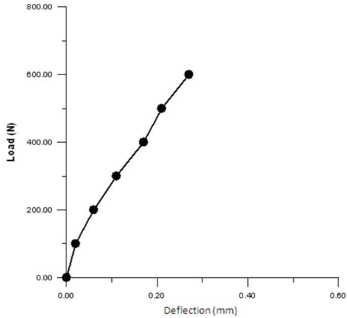
Figure (9) The load – displacement of epoxy matrix composite reinforced with 12 % wt okra fiber.
