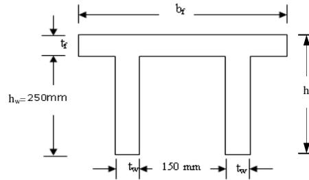
**Figure (1) Cross-Section of  $\pi$  –Beams**
