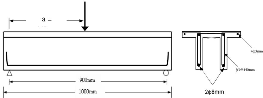
**Figure (2) Dimensions and Details of Tested  $\pi$  –Beams**
