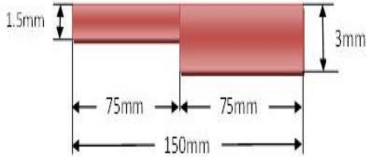
Figure (3 e) Front view of stepped thickness Plate.
