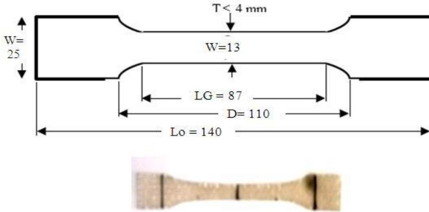
**Figure (2) Tensile specimen (All dimensions in mm).**
