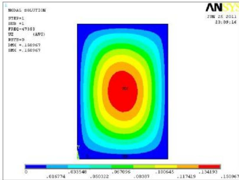
Figure (19) "Stiffened rectangular plate of biaxial load".
