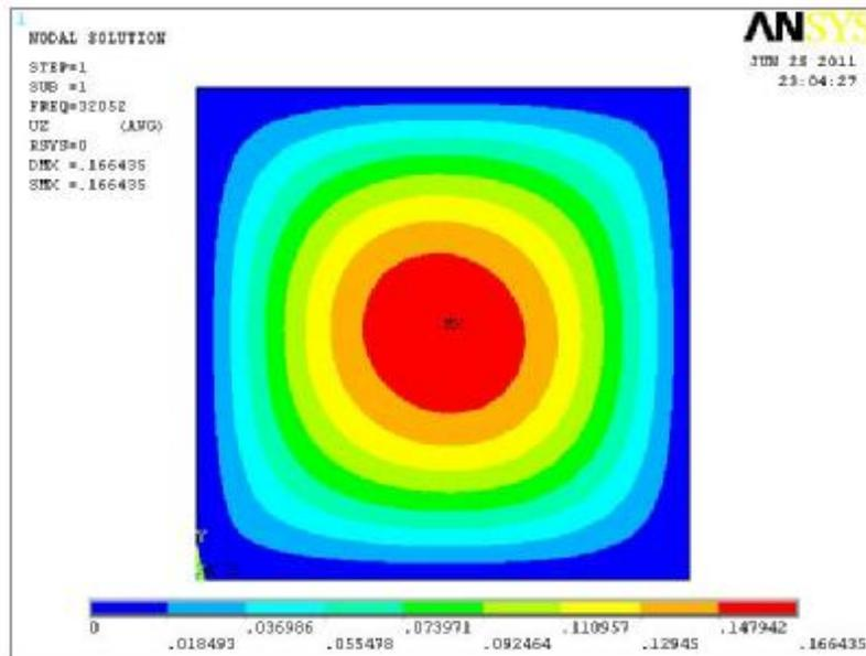
Figure (20) "Stiffened square plate of biaxial load".
