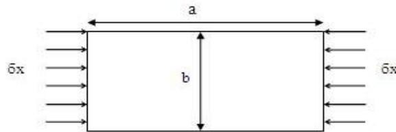
**Figure (1): Simply-supported rectangular plate under uniaxial loading.**
