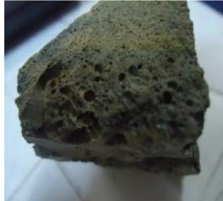
Figure(6) The created voids of sample-4
