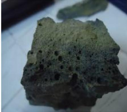
Figure(5) The created voids of sample-3
