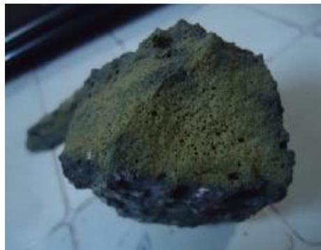
Figure(3).The created voids of sample-1
