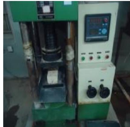
Figure(2).The compressive strength device
