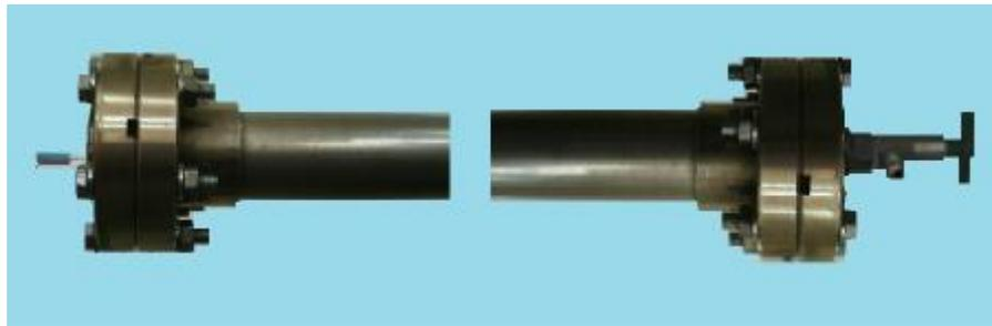
Figure (2) flanges used to close tube ends.
