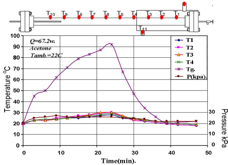
Figure (12) Variation of wall surface temperature and unit pressure, with time When the heat input is 67.2 W, adsorption pair is active carbon-acetone.
