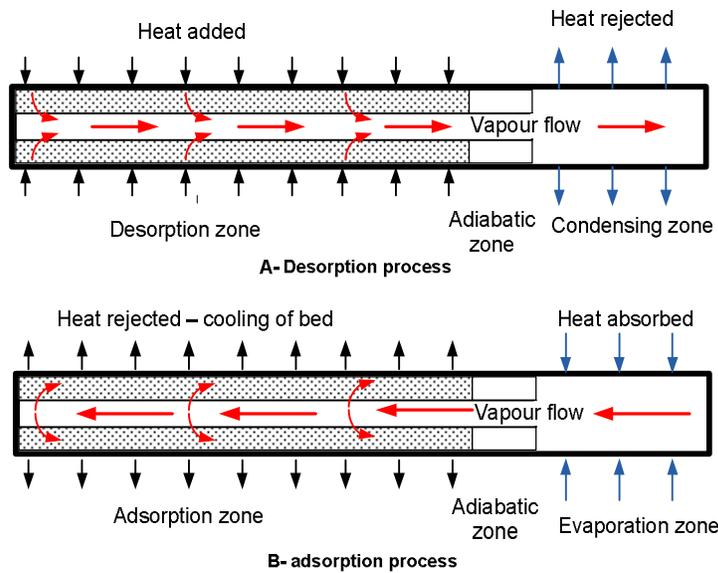
Figure (6) operation sequence of the adsorption heat pipe.
