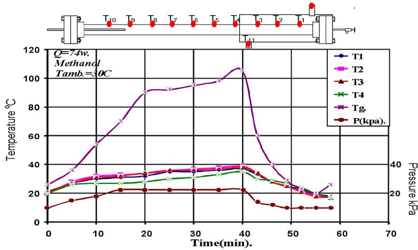
Figure (10) Variation of wall surface temperature and unit pressure, with time When the heat input is 74 W, adsorption pair is active carbon-methanol.
