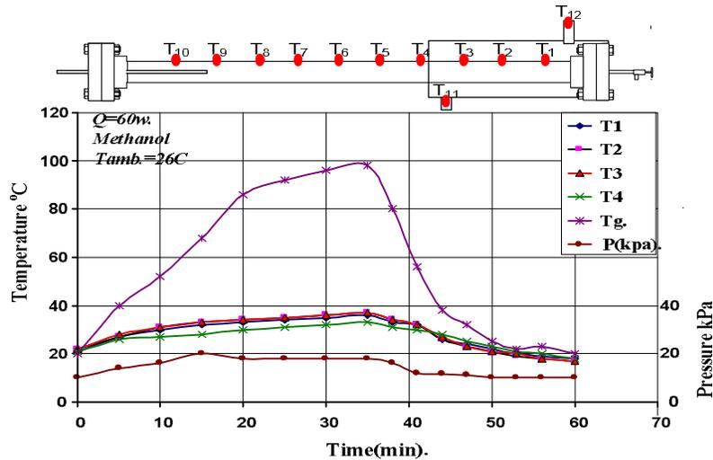
Figure (8) Variation of wall surface temperature and unit pressure, with time when the heat input is 60 W, adsorption pair is active carbon-methanol.
