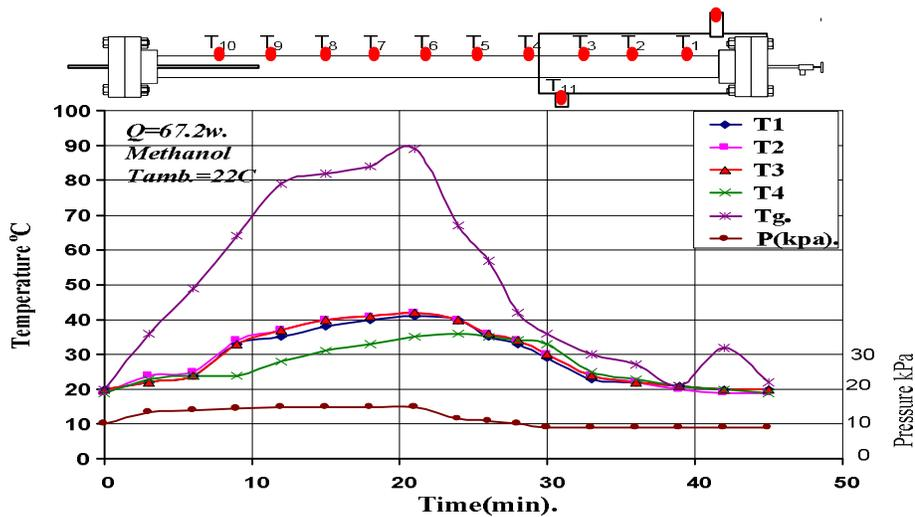
Figure (9) Variation of wall surface temperature and unit pressure, with time when the heat input is 67.2 W, adsorption pair is active carbon-methanol.
