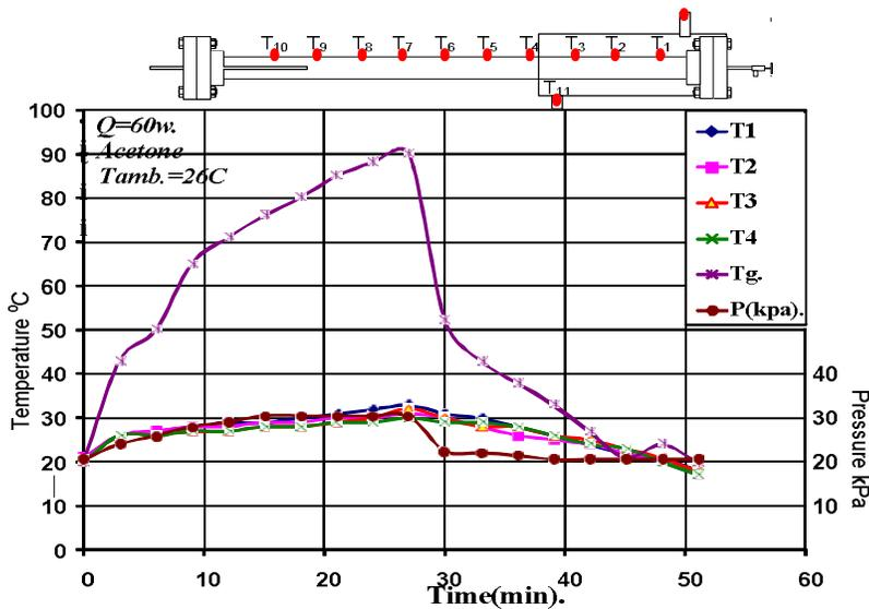
Figure (11) Variation of wall surface temperature and unit pressure, with time when the heat input is 60 W, adsorption pair is active carbon-acetone.
