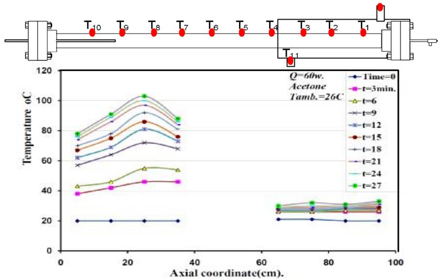
Figure (15) Variation of adsorption heat pipe wall temperatures with the axial direction and time.
