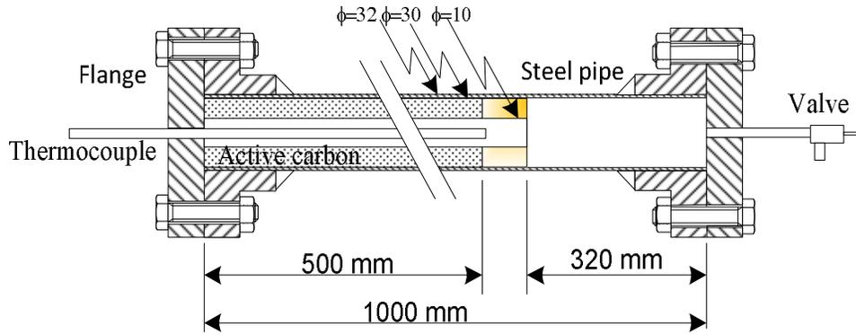
Figure (1) section in adsorption heat pipe.
