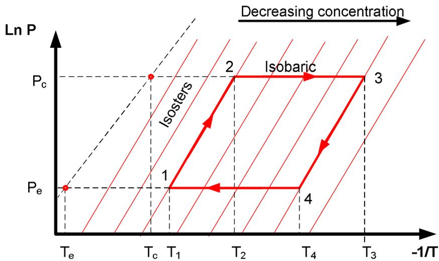
Figure (7) (P-T-x) diagram of the ideal basic adsorption cycle.
