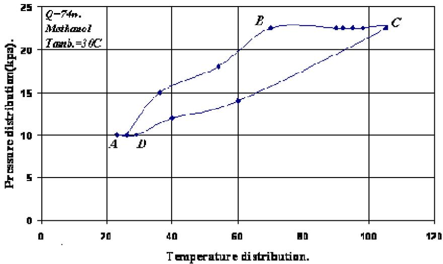
Figure (14) Adsorption cycle of the heat pipe, heat input is 74 W, active carbon-methanol pair was used.
