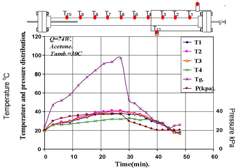
Figure (13) Variation of wall surface temperature and unit pressure, with time when the heat input is 74 W, adsorption pair is active carbon-acetone.
