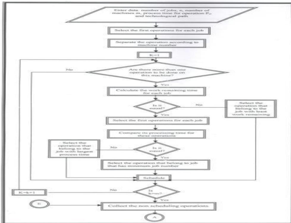
Figure (1) The logic Modified Least Work Remaining (continue)
