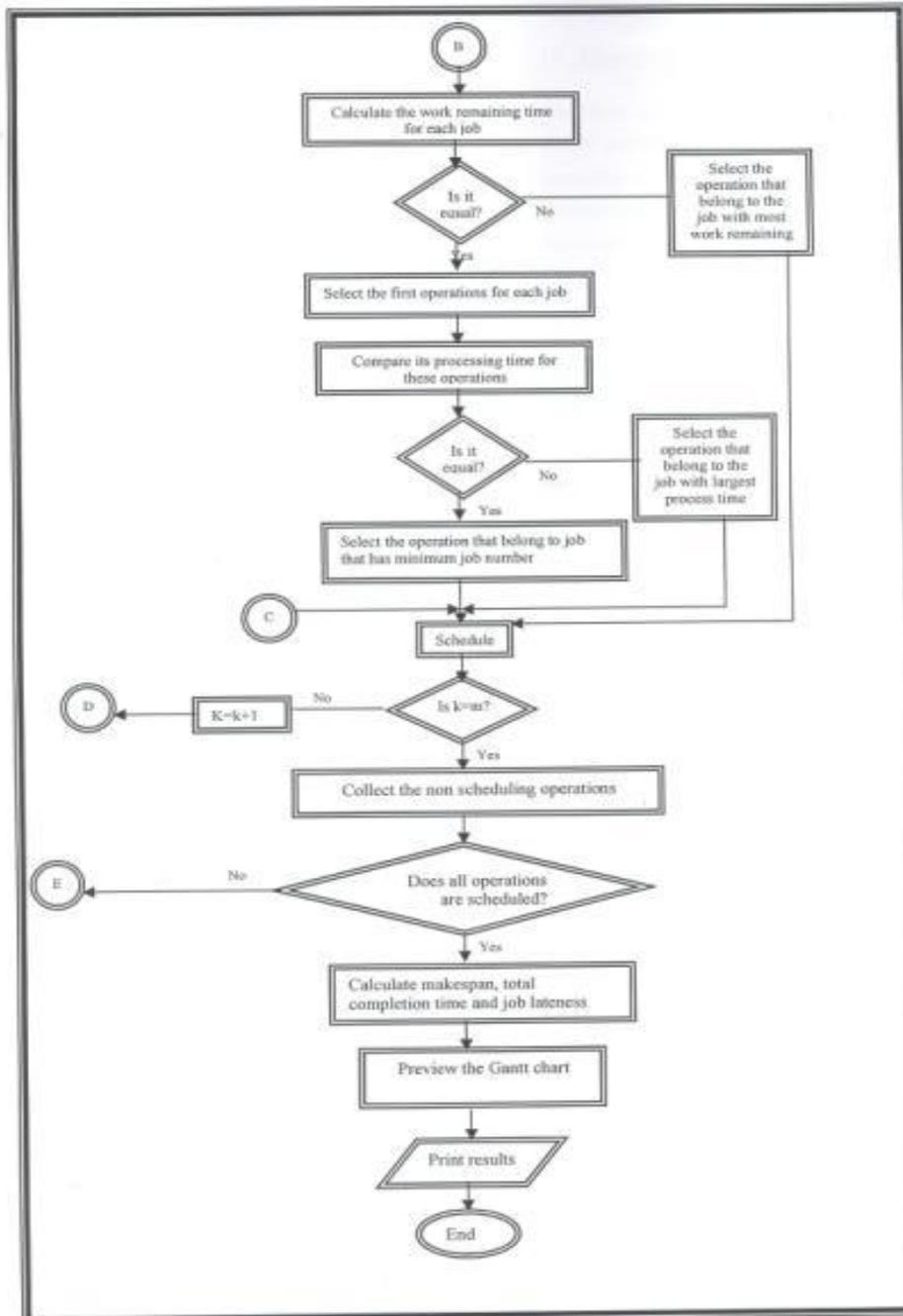
Figure (2) The logic modified Least Work Remaining .
