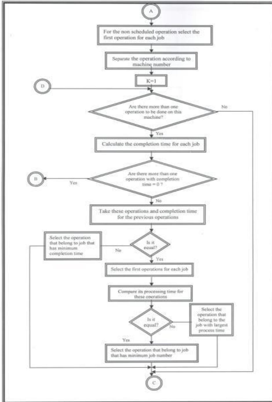
Figure (1) The logic Modified Least Work Remaining (continue).
