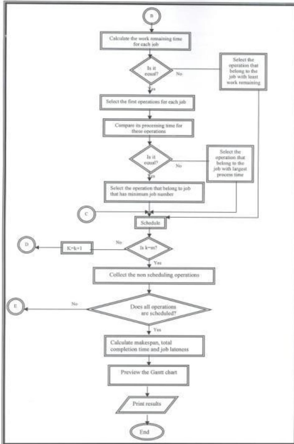
Figure (1) The logic modified Least Work Remaining .
