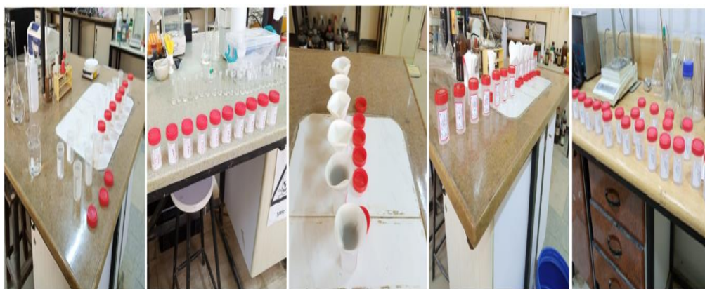
Figure 5: The process of filtration for chromium solution from glass sand after the process of sorption
