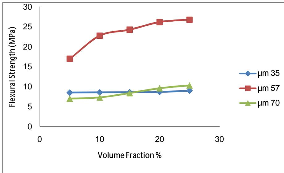
Figure (2): The flexural strength for mica filled UP composites with different filler loading.
