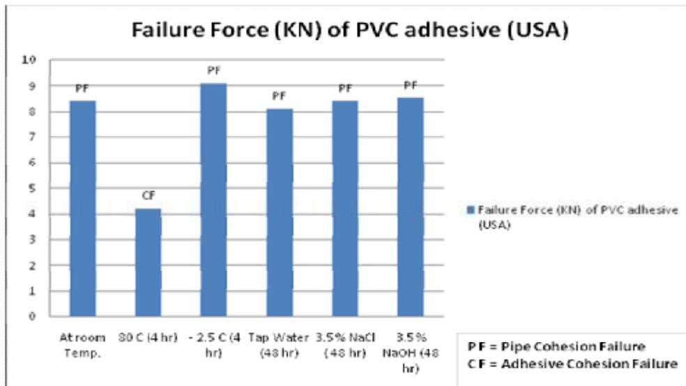
Figure (6) show results of pipe adhesion testing for PVC pipe with PVC adhesive (USA) with surface treatment, under environmental conditions.
