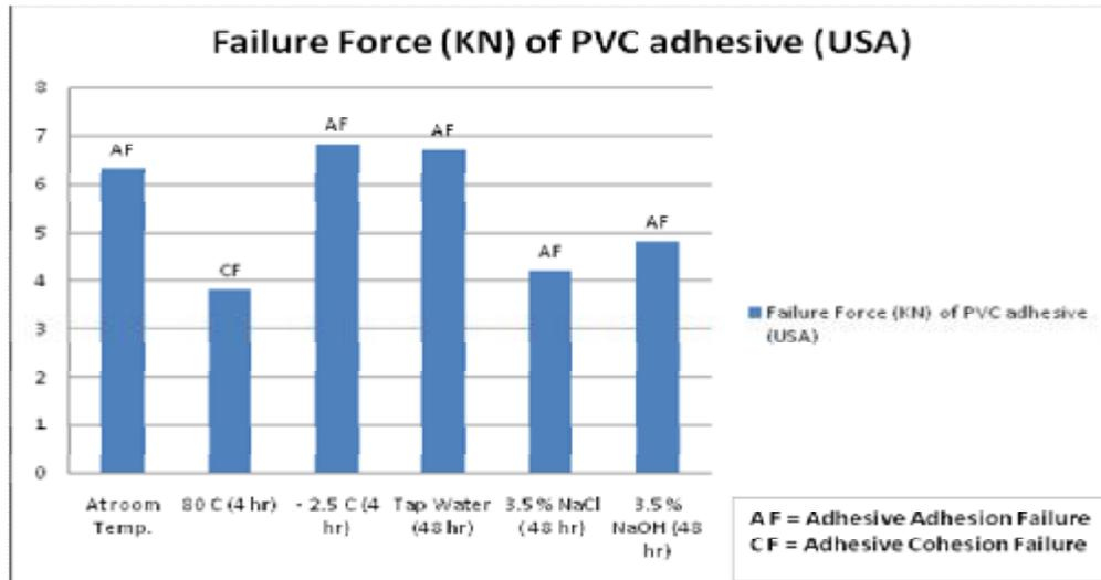
Figure (3) show results of pipe adhesion testing for PVC pipe with PVC adhesive (USA) without surface treatment, under environmental conditions.
