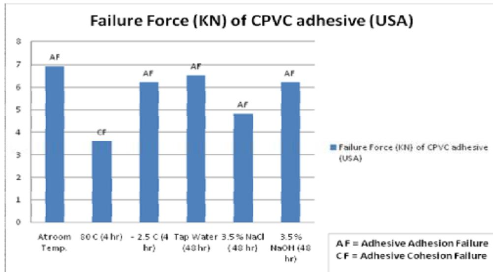
Figure (4) show results of pipe adhesion testing for PVC pipe with CPVC adhesive (USA) without surface treatment, under environmental conditions.
