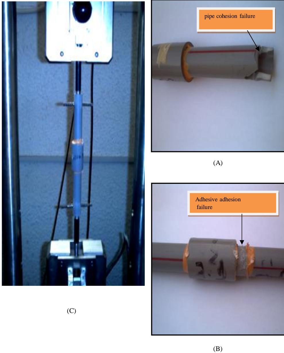
Figure (2) (A, B, C) Appearance of samples of PVC pipe adhesion testing.
