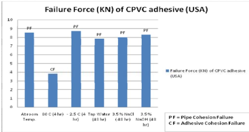
Figure (7) show results of pipe adhesion testing for PVC pipe with CPVC adhesive (USA) with surface treatment, under environmental conditions.
