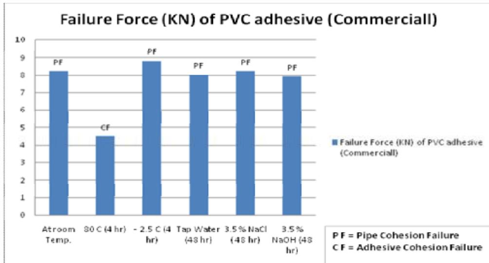
Figure (8) show results of pipe adhesion testing for PVC pipe with PVC adhesive (Commercial) with surface treatment, under environmental conditions.
