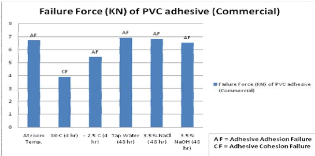
Figure (5) show results of pipe adhesion testing for PVC pipe with PVC adhesive (Commercial) without surface treatment, under environmental conditions.
