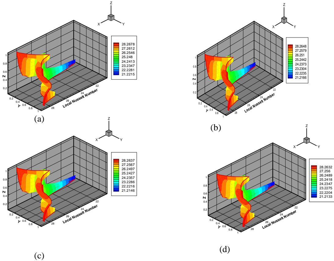
Figure (7) Local Nu contour for hot wall,  $\Omega=50$  rad/s : (a)  $\Delta T = 100$ ,  $Ra=1.19*10^8$ ,  $Ra_r = 2.88*10^{10}$  (b)  $\Delta T = 200$ ,  $Ra=2.09*10^8$ ,  $Ra_r = 5.08*10^{10}$  (c)  $\Delta T = 300$ ,  $Ra=2.81*10^8$ ,  $Ra_r = 6.81*10^{10}$  (d)  $\Delta T = 400$ ,  $Ra=3.39*10^8$ ,  $Ra_r = 8.21*10^{10}$ .
