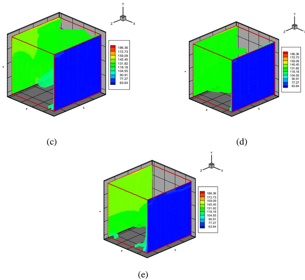
Figure (4) Temperature contour  $Ra=1.67 * 10^8$ ,  $\Delta T = 150$  : (a)  $\Omega=0$ , (b)  $\Omega=10$  rad/s,  $Ra_r = 1.6 * 10^9$ , (c)  $\Omega=20$  rad/s,  $Ra_r = 6.47 * 10^9$ , (d)  $\Omega=30$  rad/s,  $Ra_r = 1.46 * 10^{10}$ , (e)  $\Omega=40$  rad/s,  $Ra_r = 2.59 * 10^{10}$ .
