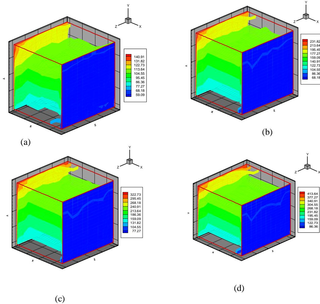
**Figure (5) Temperature contour,  $\Omega = 50$  rad/s: (a)  $\Delta T = 100$ ,  $Ra = 1.19 * 10^8$ ,  $Ra_r = 2.88 * 10^{10}$  (b)  $\Delta T = 200$ ,  $Ra = 2.09 * 10^8$ ,  $Ra_r = 5.08 * 10^{10}$  (c)  $\Delta T = 300$ ,  $Ra = 2.81 * 10^8$ ,  $Ra_r = 6.81 * 10^{10}$  (d)  $\Delta T = 400$ ,  $Ra = 3.39 * 10^8$ ,  $Ra_r = 8.21 * 10^{10}$ .**
