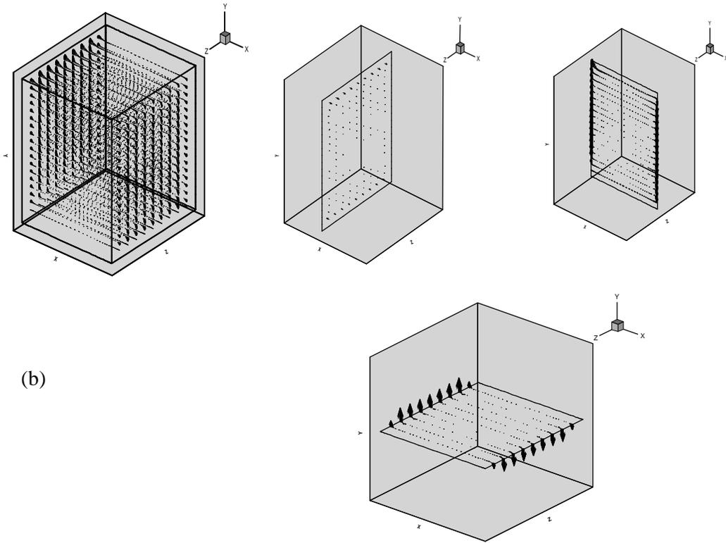
Figure (3) Velocity vector: (a)  $\Omega = 20$  rad/s,  $Ra=1.67*10^{10}$ ,  $Ra_r=6.47*10^{11}$ , scale=0.1 relative to grid units/magnitude, (b)  $\Omega = 0$ ,  $Ra=1.67*10^{10}$ , scale=0.2 relative to grid units/magnitude.
