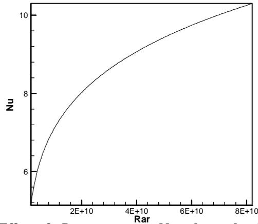
Figure (8) Effect of  $Ra_r$  on average Nusselt number  $Nu$  for different temperature difference  $\Delta T$  and different angular velocities of enclosure  $\Omega$ .
