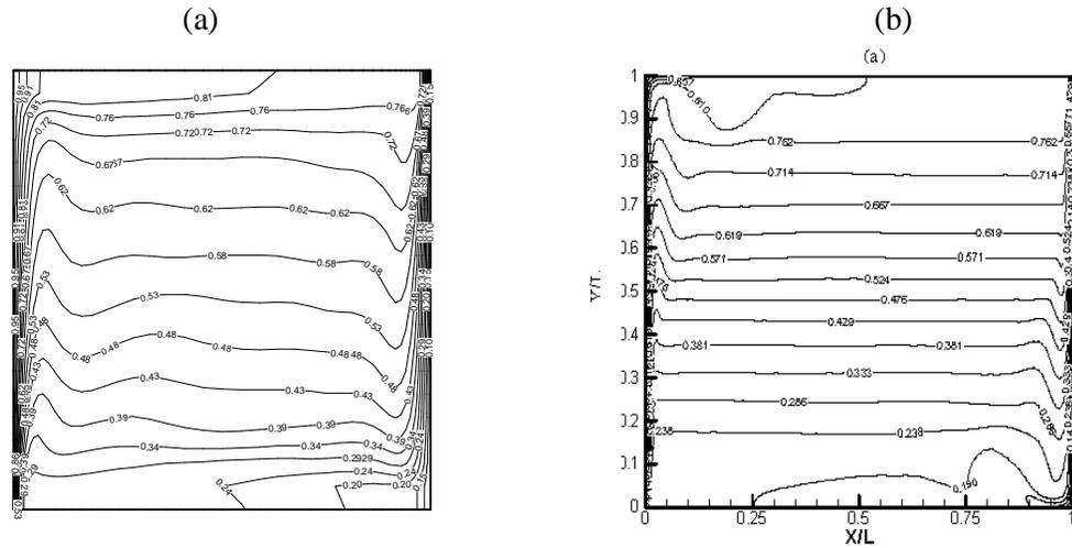
Figure (2) Comparison of the temperature contours for (a) present numerical results, (b) previous work by Bouaraour[7] with  $(Ra = 1.58 * 10^9)$ .
