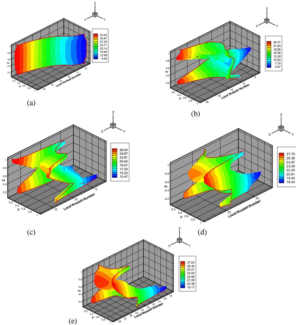
Figure (6) Local Nu contour for hot wall  $Ra=1.67 \times 10^8$ ,  $\Delta T = 150$  : (a)  $\Omega=0$ , (b)  $\Omega=10$  rad/s,  $Ra_r = 1.6 \times 10^9$ , (c)  $\Omega=20$  rad/s,  $Ra_r = 6.47 \times 10^9$ , (d)  $\Omega=30$  rad/s,  $Ra_r = 1.46 \times 10^{10}$ , (e)  $\Omega=40$  rad/s,  $Ra_r = 2.59 \times 10^{10}$ .
