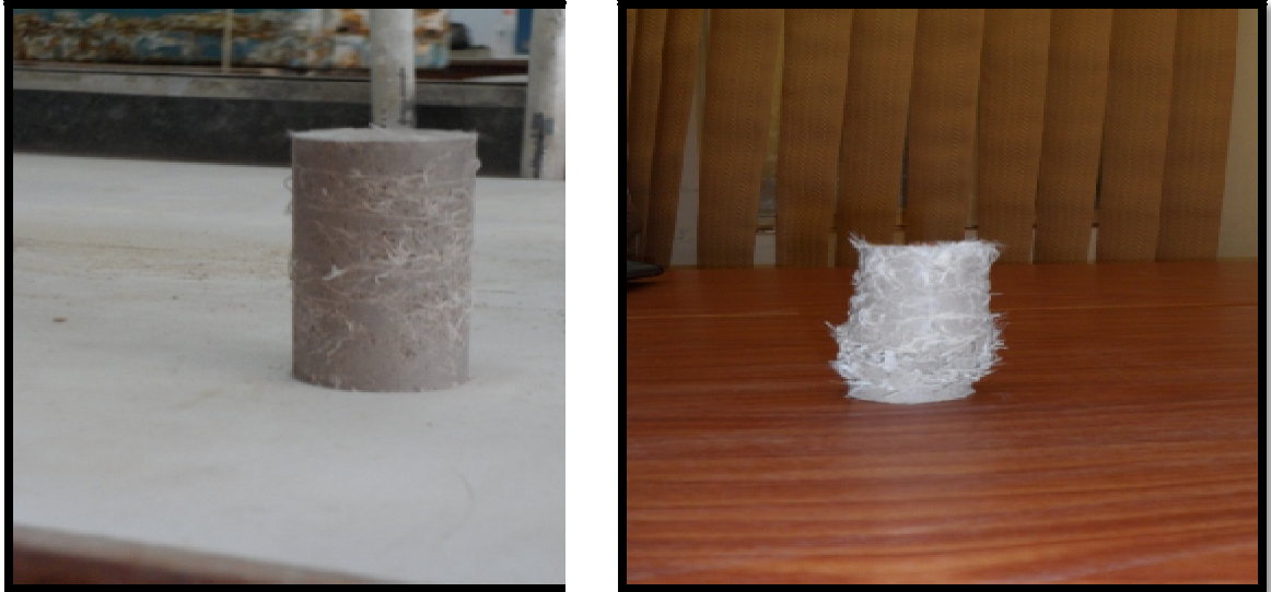
Figure (11): failure sample before and after the unconfined compression test.
